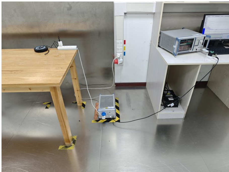
Measurement of Conducted Emissions Test Set Up
