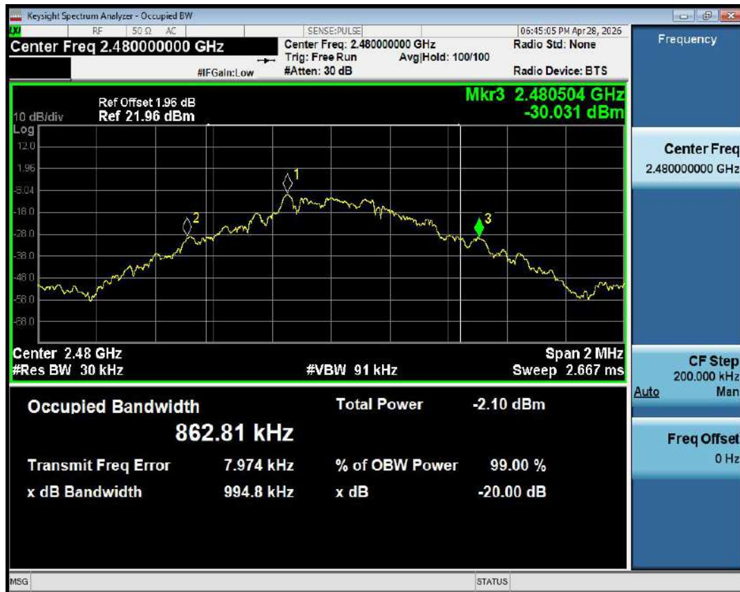
-20dB Bandwidth NVNT 1-DH1 2480MHz Ant1
