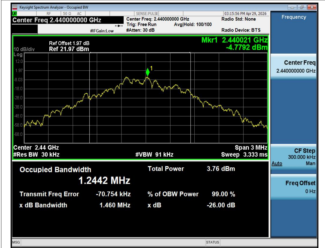
OBW NVNT GFSK 2440MHz Ant1
