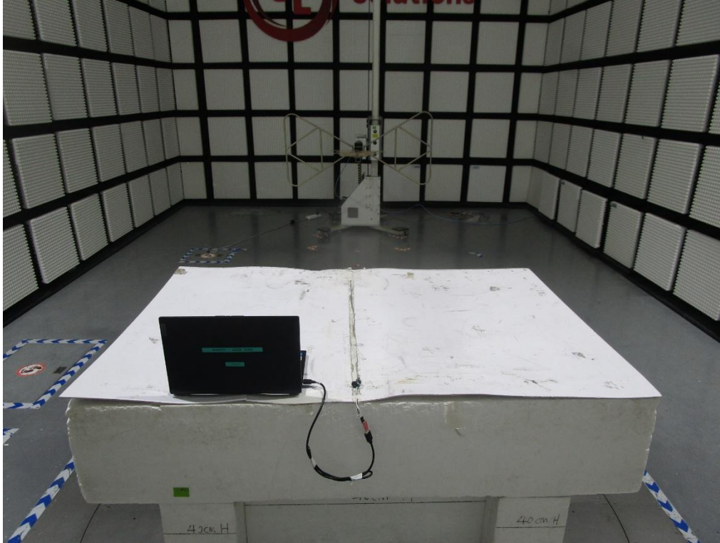
RADIATED RF MEASUREMENT SETUP (Below 30MHz)
