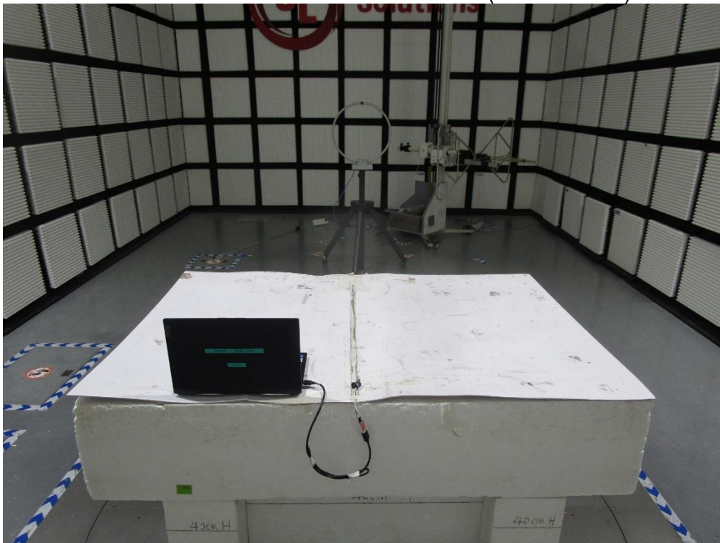
RADIATED RF MEASUREMENT SETUP (Below 30MHz)
