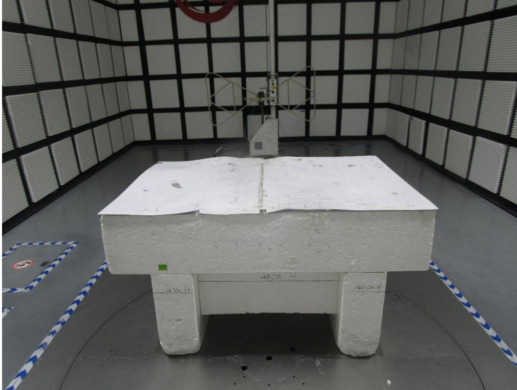
RADIATED RF MEASUREMENT SETUP (Below 30MHz)
