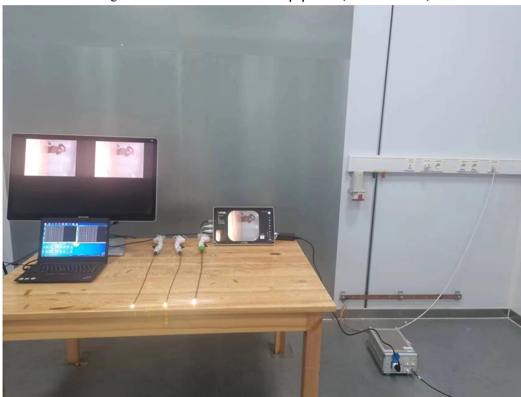
Fig. 4 Power line conducted emission setup photo
