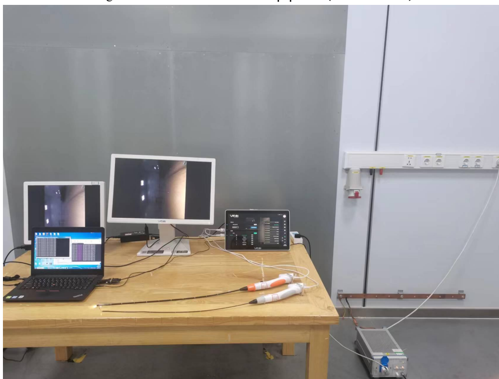
Fig. 4 Power line conducted emission setup photo
