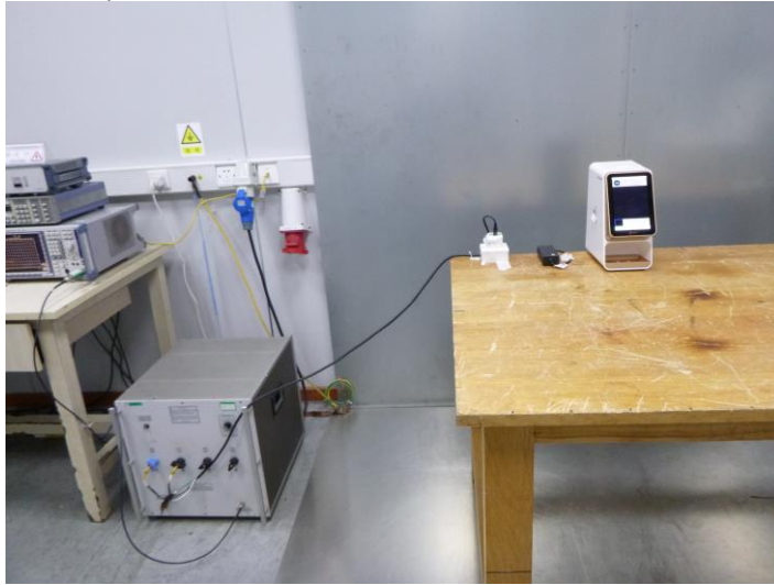
Radiated Emissions (30MHz-1GHz)
