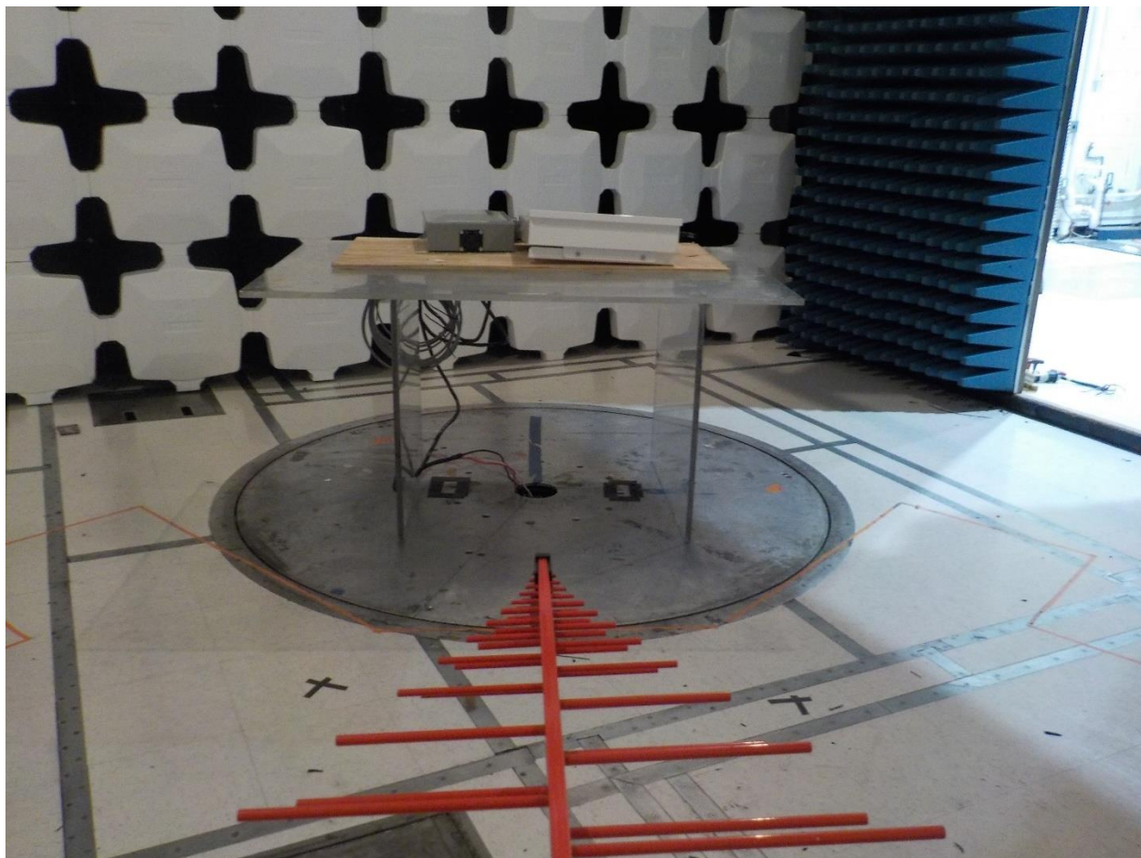
Figure 2: REE Setup (30MHz-1GHz)
