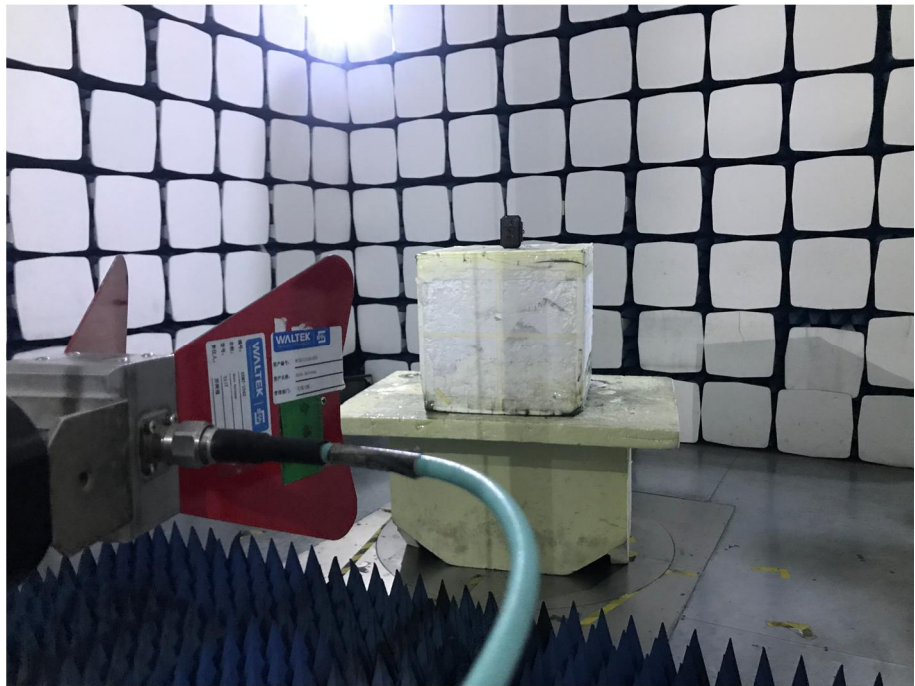
Radiation Emission Test Setup (1GHz to 18GHz)
