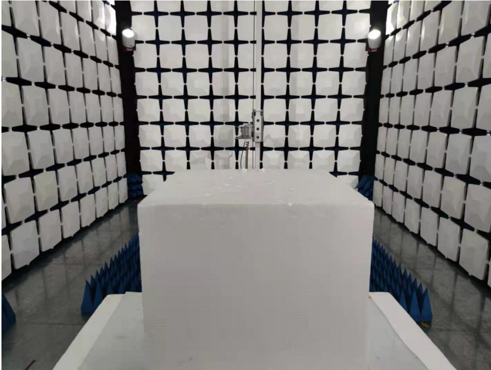
Above 1GHz for radiated emission test setup
