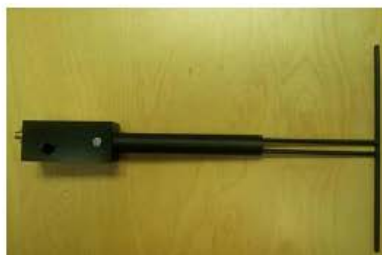
Figure 1 – MVG COMOSAR Validation Dipole
