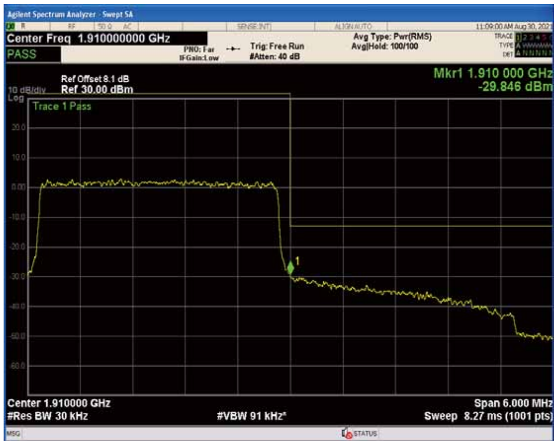
Band2 QAM16 BW=3MHz Channel=19185 RB Size=1 Position=#0
