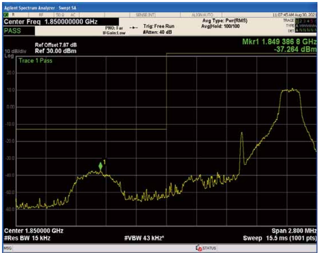
Band2 QPSK BW=1.4MHz Channel=19193 RB Size=1 Position=#0
