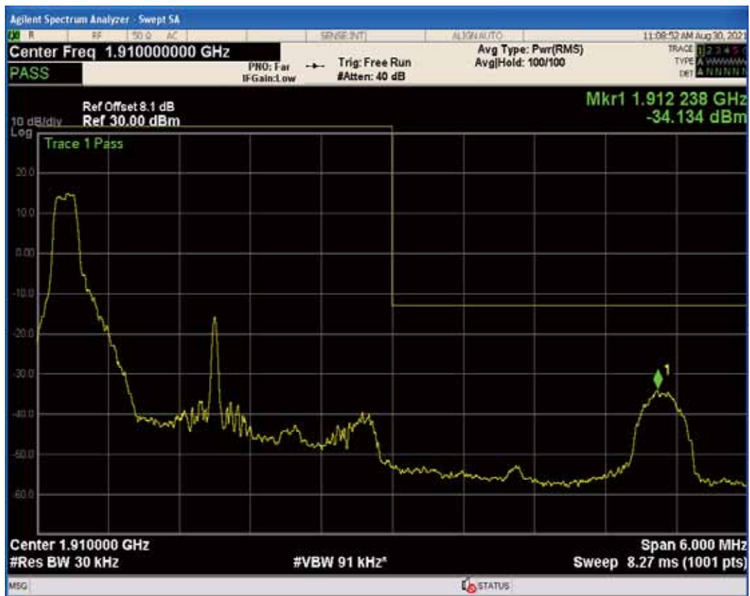
Band2 QPSK BW=3MHz Channel=19185 RB Size=1 Position=#Max
