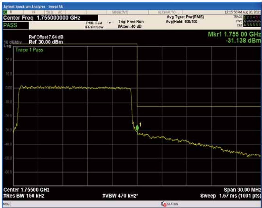
Band4 QPSK BW=20MHz Channel=20050 RB Size=1 Position=#Max
