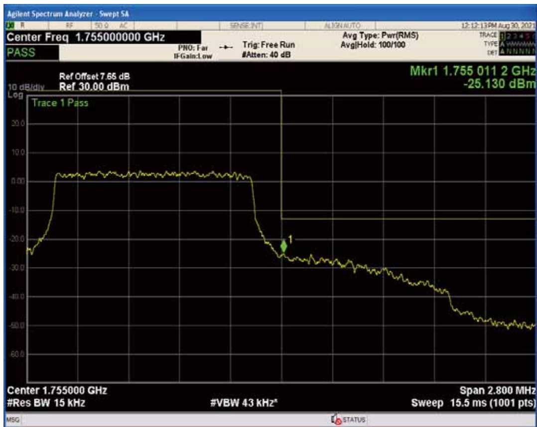
Band4 QAM16 BW=1.4MHz Channel=20393 RB Size=1 Position=#0
