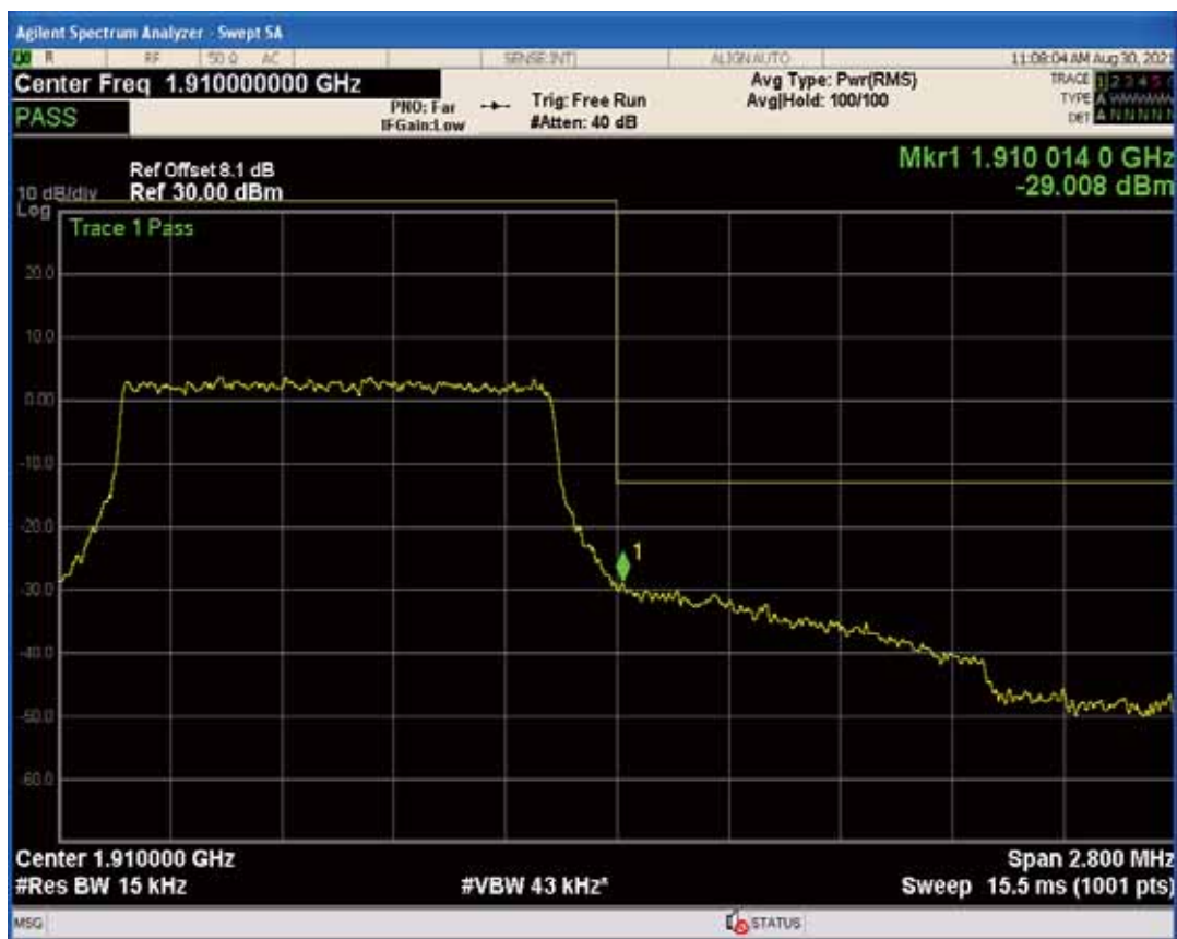
Band2 QAM16 BW=1.4MHz Channel=19193 RB Size=1 Position=#0
