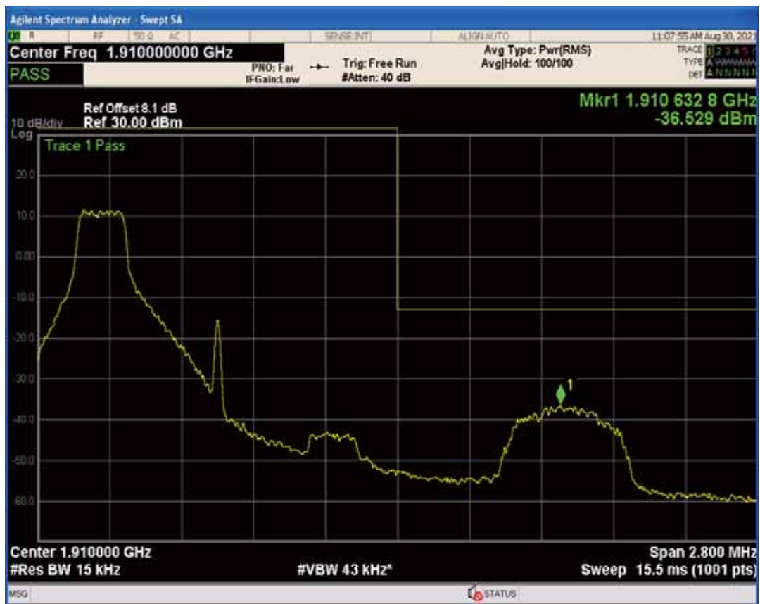
Band2 QPSK BW=1.4MHz Channel=19193 RB Size=1 Position=#Max
