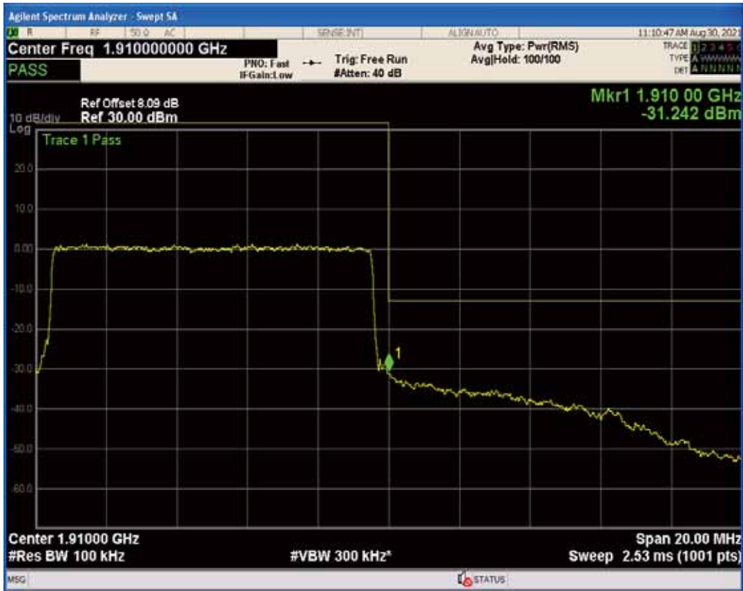
Band2 QPSK BW=15MHz Channel=18675 RB Size=1 Position=#Max
