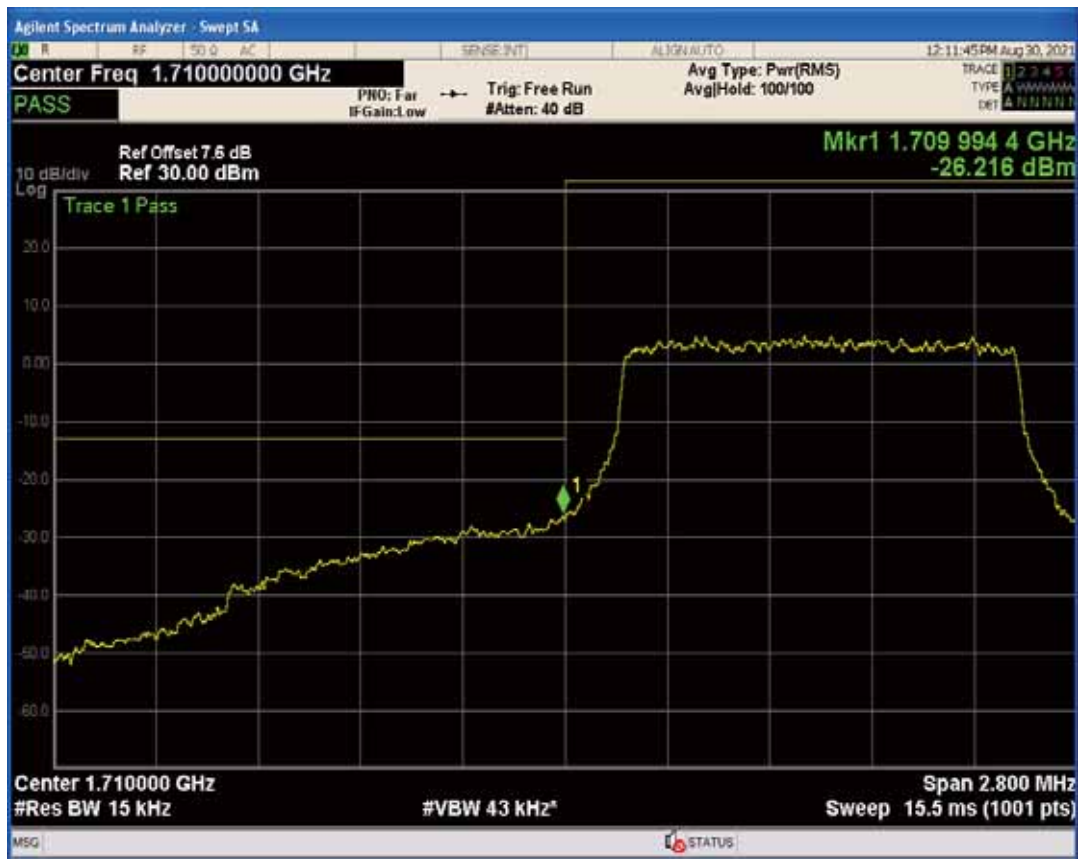
Band4 QAM16 BW=1.4MHz Channel=19957 RB Size=1 Position=#Max
