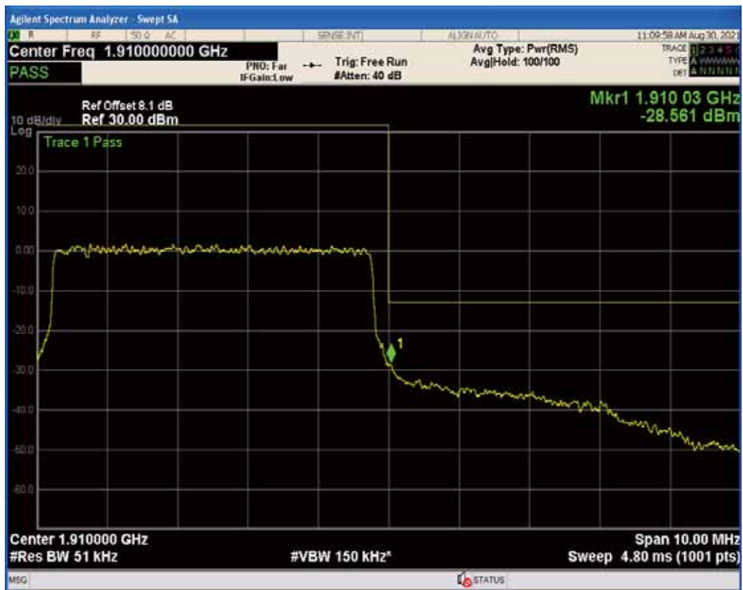
Band2 QAM16 BW=5MHz Channel=19175 RB Size=1 Position=#Max
