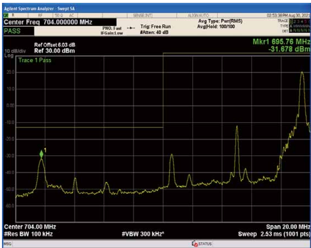
Band17 QPSK BW=10MHz Channel=23780 RB Size=1 Position=#0
