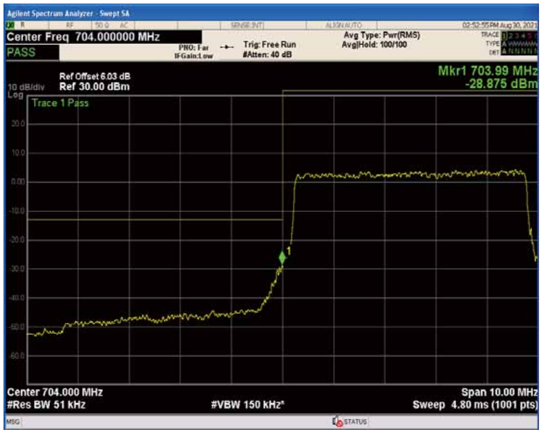
Band17 QPSK BW=5MHz Channel=23755 RB Size=1 Position=#Max
