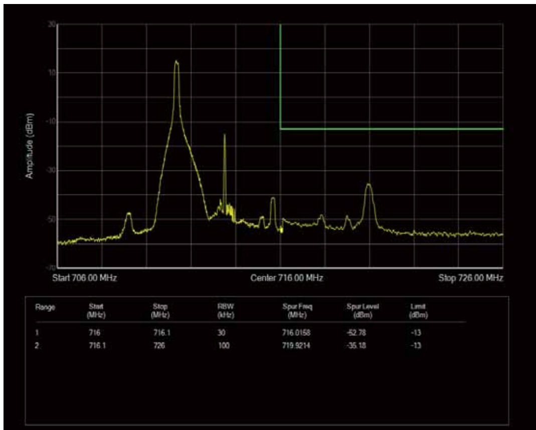
Band12 QPSK BW=10MHz Channel=23060 RB Size=1 Position=#0
