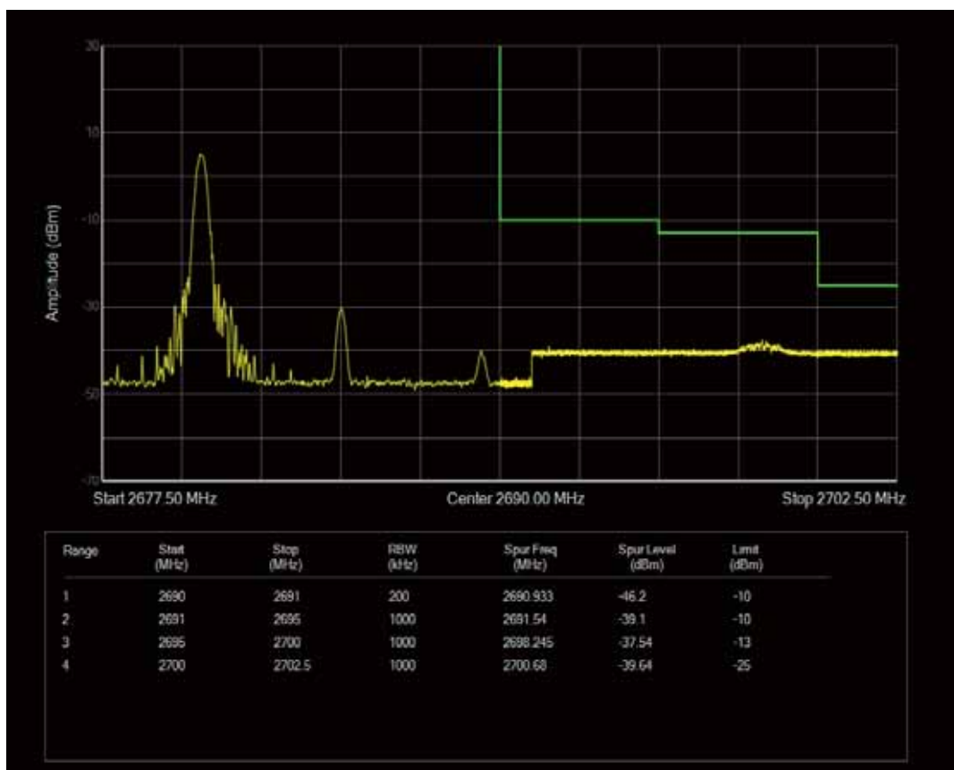
Band41 QAM16 BW=10MHz Channel=41540 RB Size=1 Position=#Max
