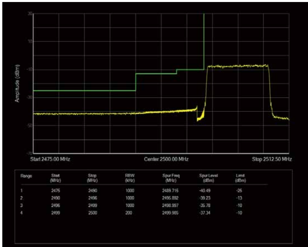
Band7 QPSK BW=10MHz Channel=20800 RB Size=1 Position=#Max
