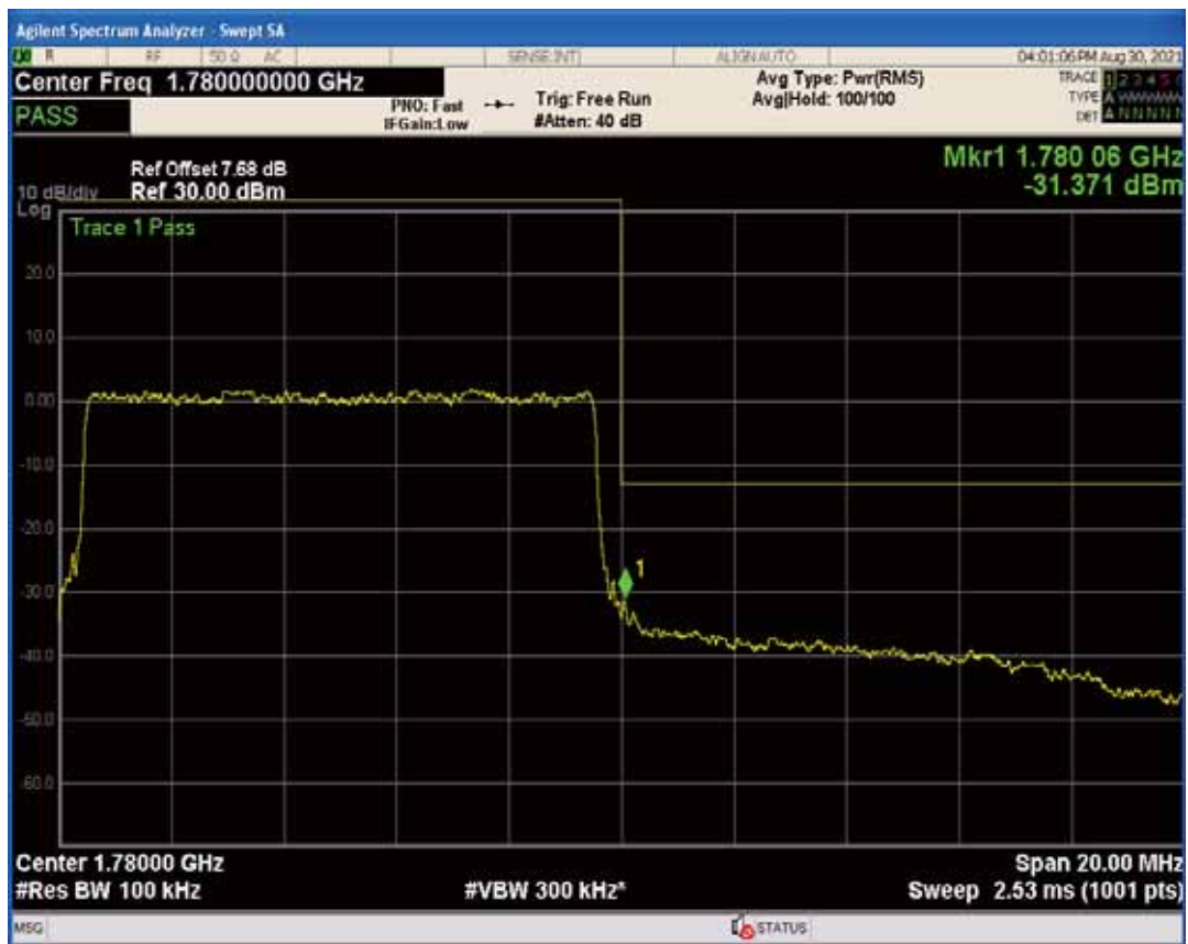
Band66 QPSK BW=15MHz Channel=132047 RB Size=1 Position=#Max
