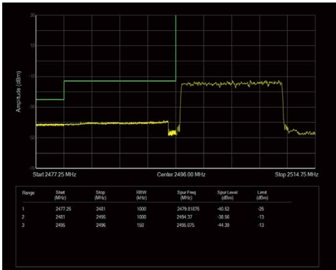
Band41 QAM16 BW=15MHz Channel=39725 RB Size=1 Position=#0
