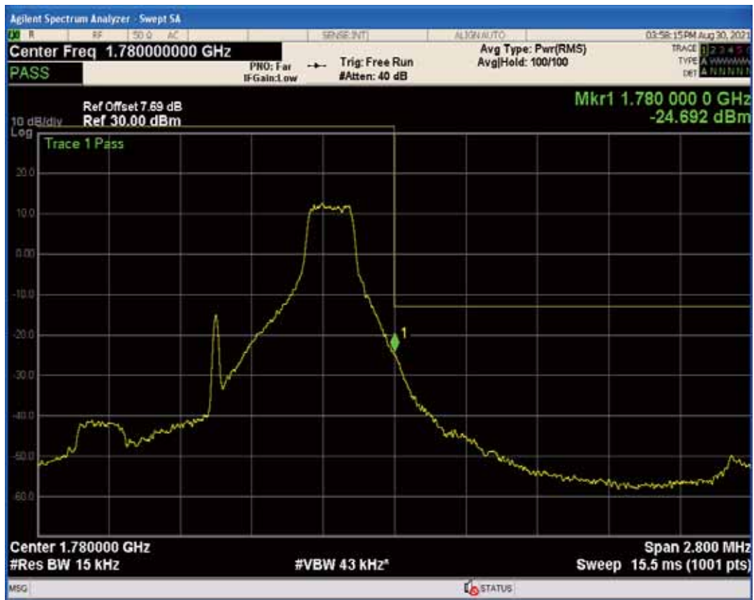
Band66 QPSK BW=1.4MHz Channel=132665 RB Size=6 Position=#0
