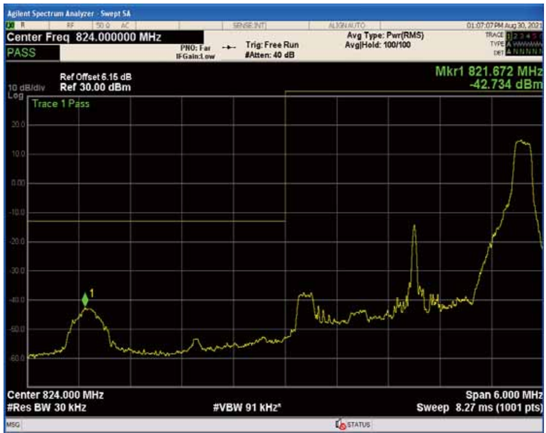
Band5 QAM16 BW=3MHz Channel=20415 RB Size=1 Position=#0
