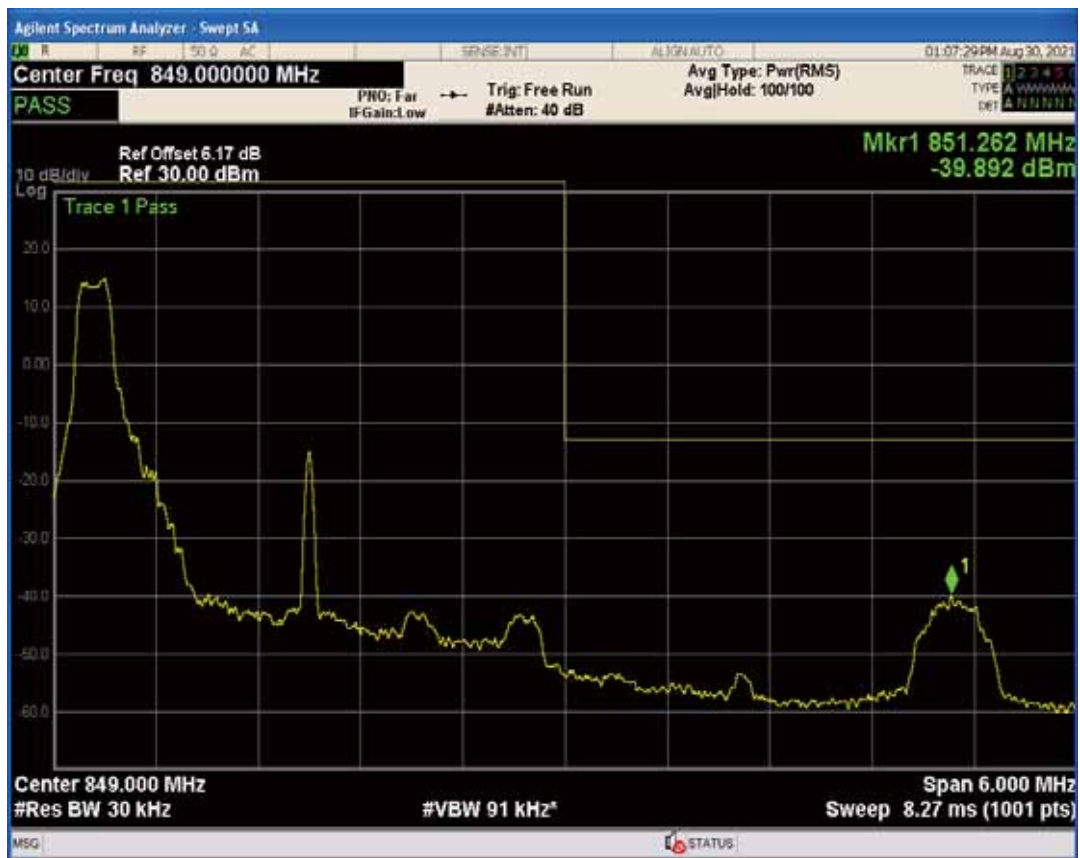
Band5 QAM16 BW=3MHz Channel=20635 RB Size=15 Position=#0
