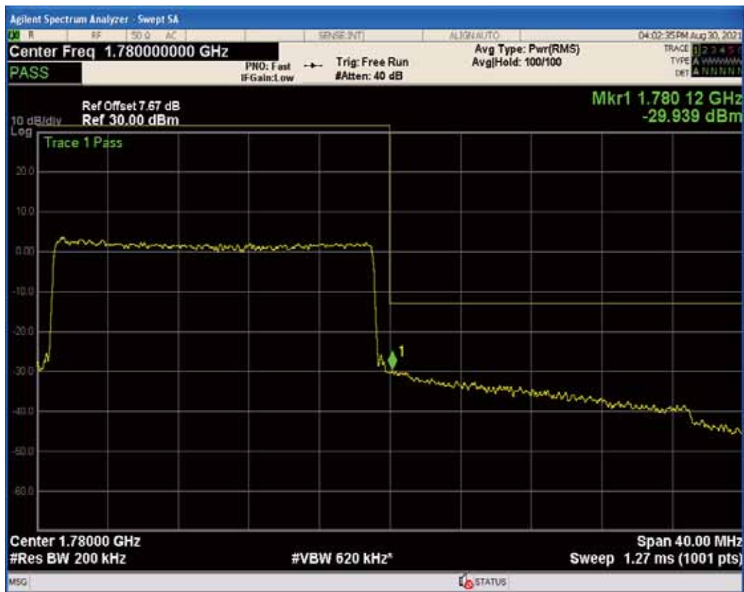
Band66 QAM16 BW=20MHz Channel=132572 RB Size=1 Position=#Max
