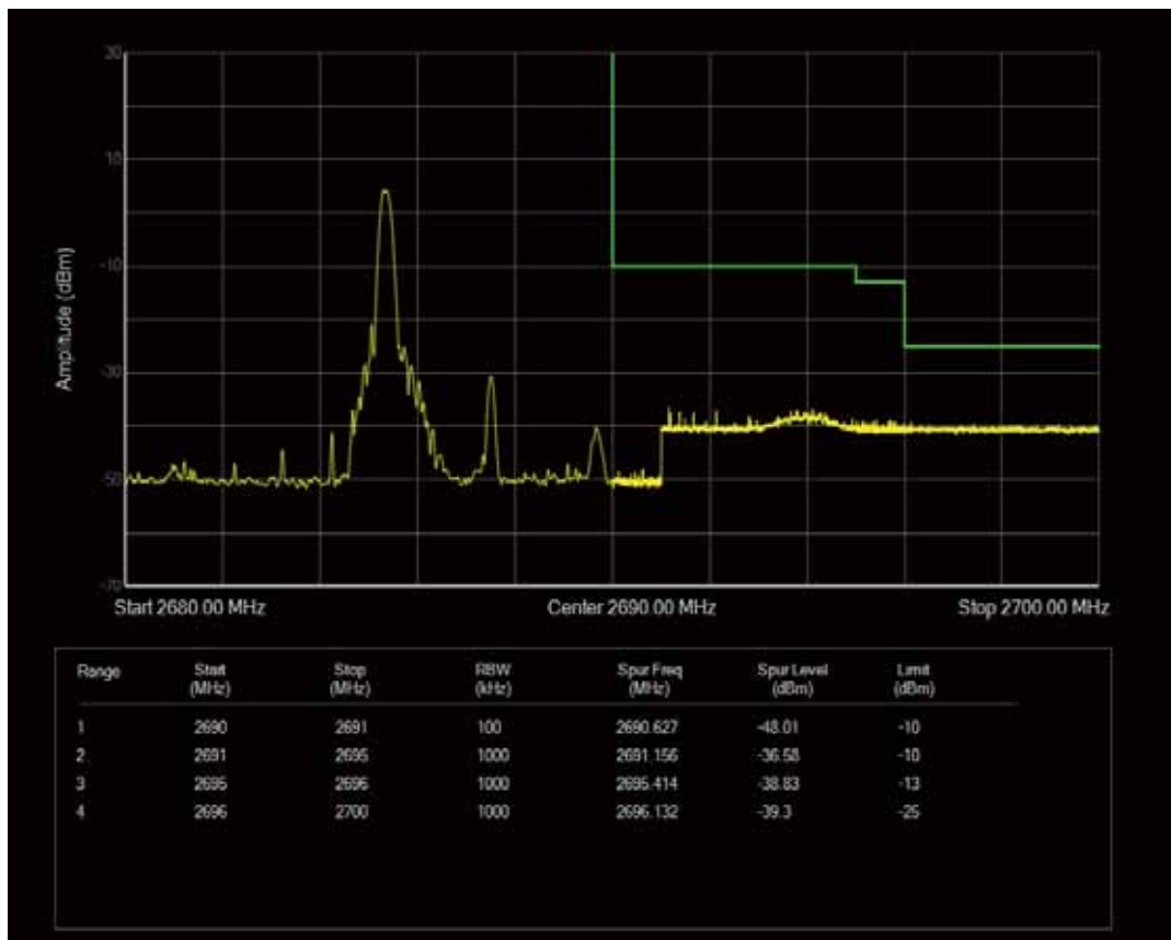
Band41 QPSK BW=5MHz Channel=41565 RB Size=1 Position=#Max
