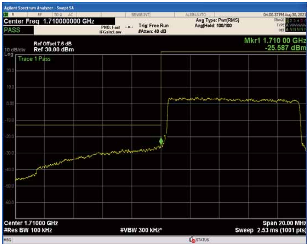
Band66 QAM16 BW=10MHz Channel=132022 RB Size=1 Position=#Max
