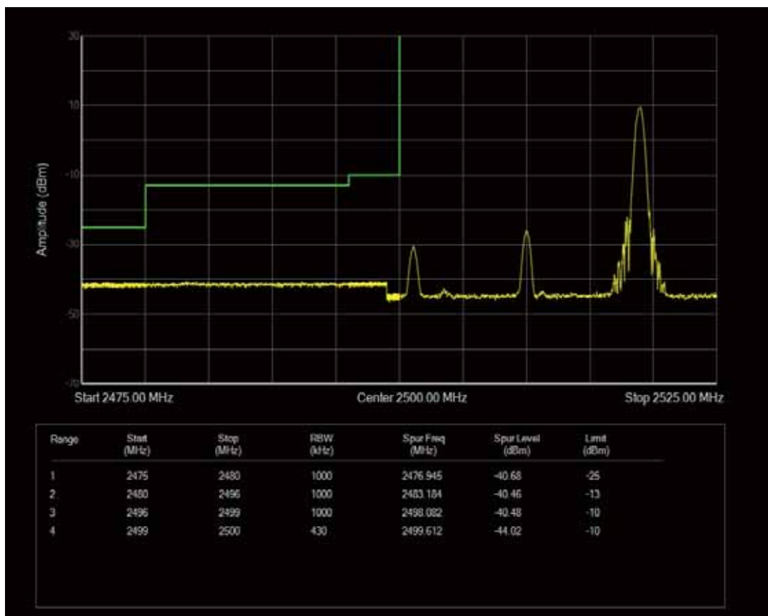
Band7 QPSK BW=20MHz Channel=20850 RB Size=1 Position=#0
