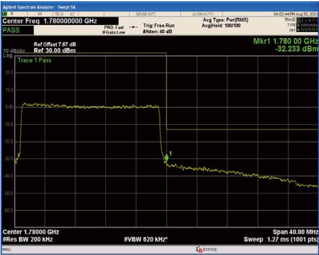
Band7 QPSK BW=5MHz Channel=20775 RB Size=1 Position=#0
