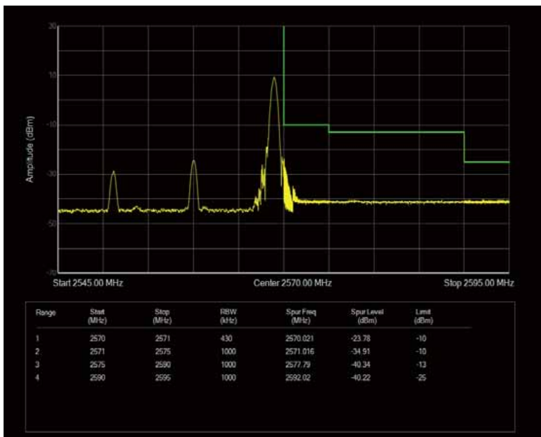
Band71 QPSK BW=5MHz Channel=133147 RB Size=1 Position=#0
