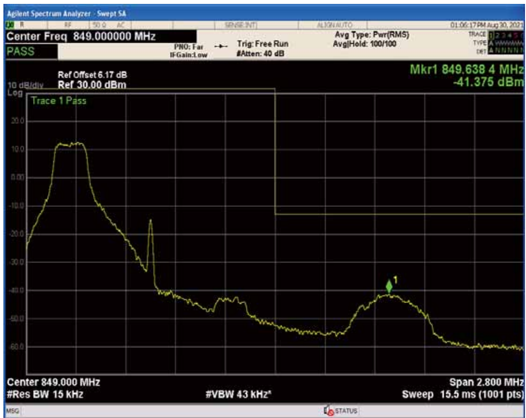
Band5 QPSK BW=1.4MHz Channel=20643 RB Size=1 Position=#Max
