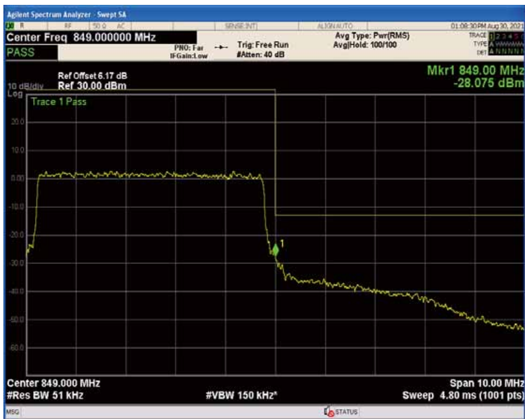
Band5 QAM16 BW=5MHz Channel=20625 RB Size=1 Position=#Max
