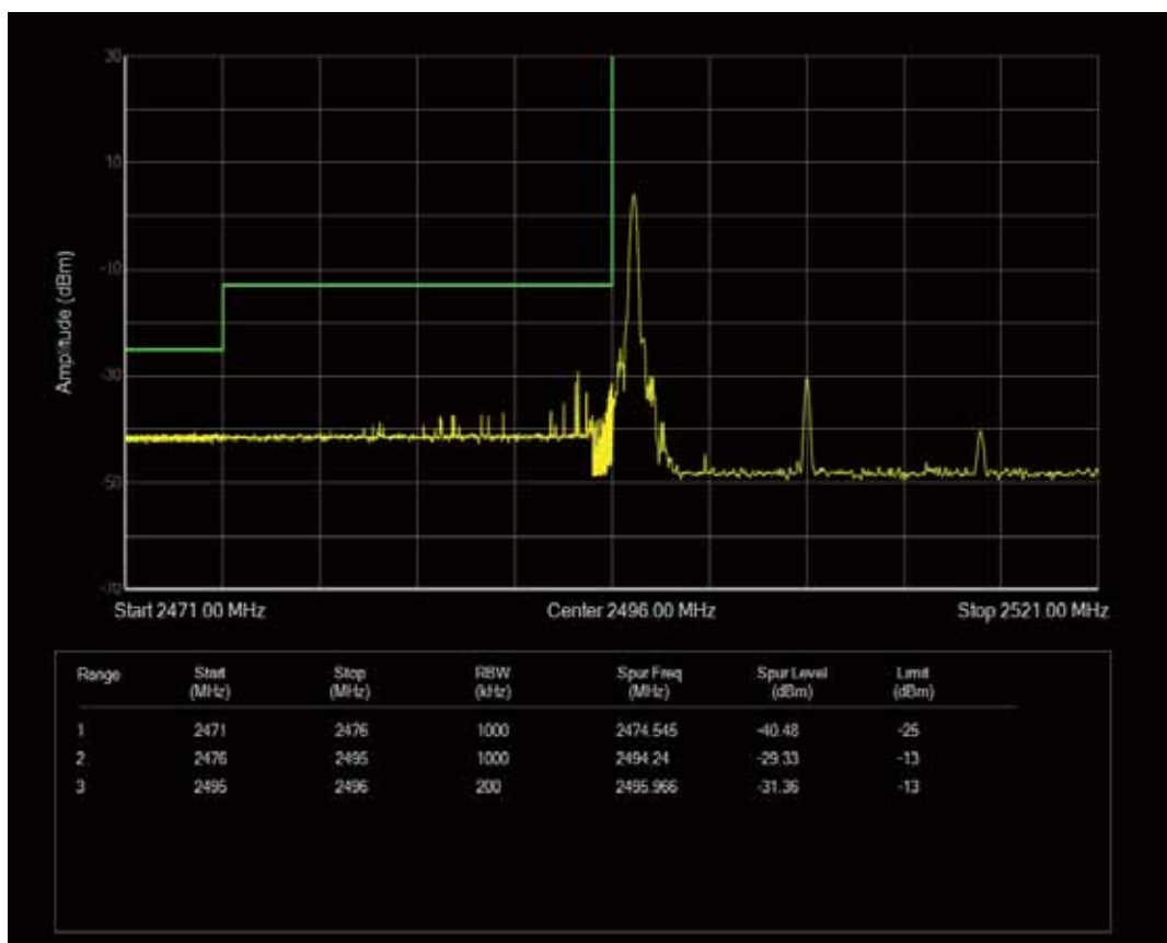
Band41 QAM16 BW=20MHz Channel=39750 RB Size=100 Position=#0
