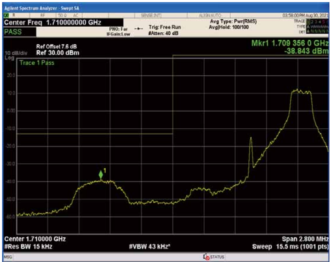
Band66 QPSK BW=1.4MHz Channel=132665 RB Size=1 Position=#0
