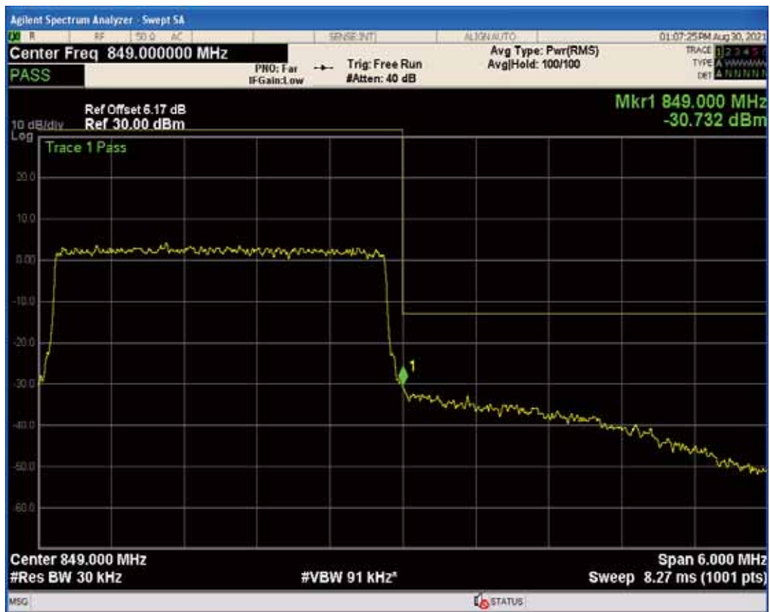
Band5 QAM16 BW=3MHz Channel=20635 RB Size=1 Position=#Max
