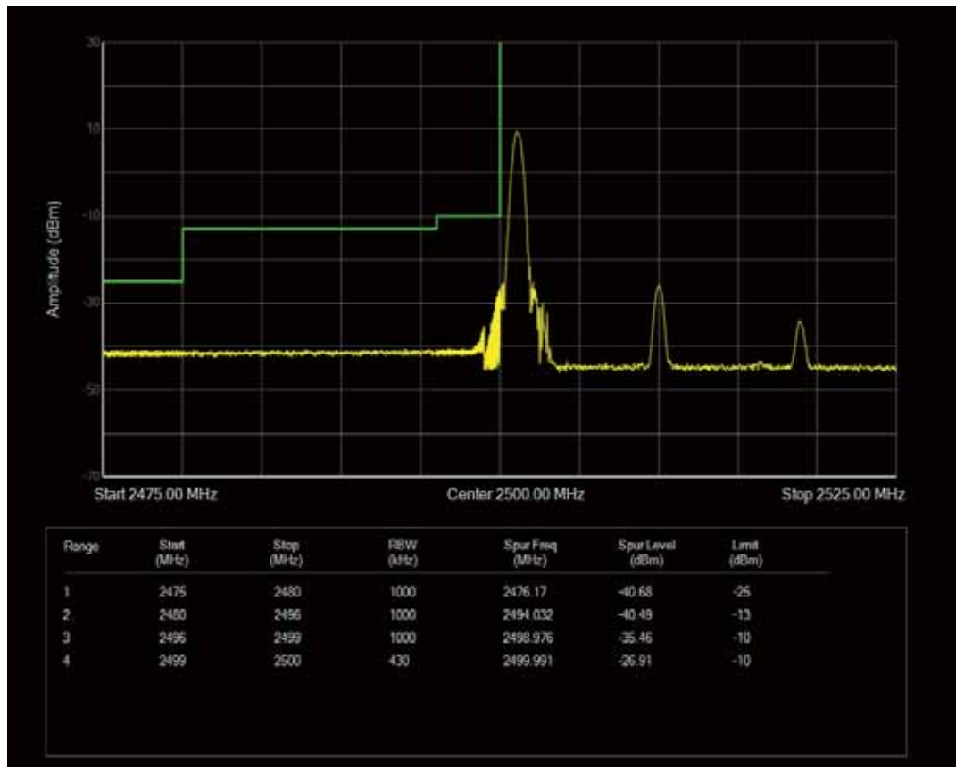
Band7 QPSK BW=20MHz Channel=20850 RB Size=100 Position=#0
