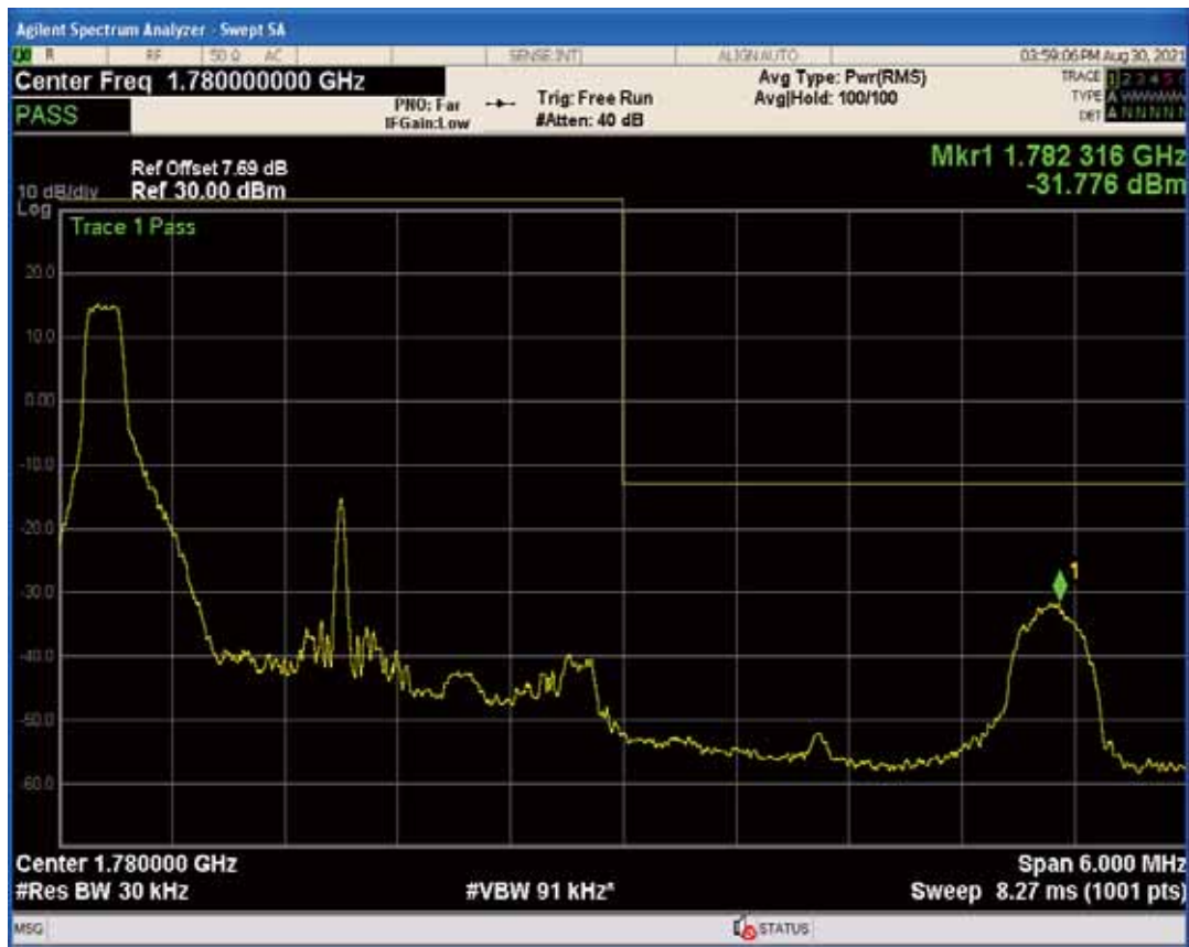
Band66 QAM16 BW=3MHz Channel=131987 RB Size=15 Position=#0
