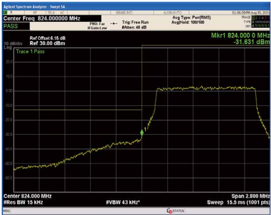
Band5 QPSK BW=1.4MHz Channel=20643 RB Size=1 Position=#0
