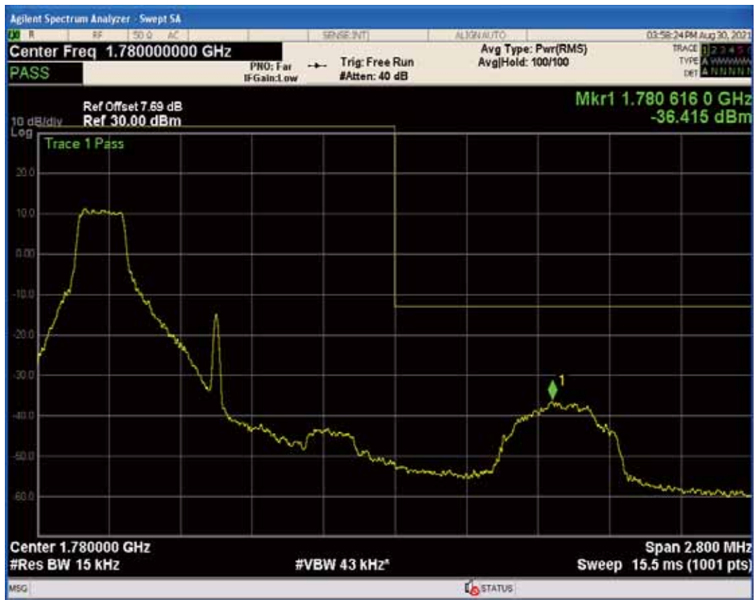
Band66 QAM16 BW=1.4MHz Channel=132665 RB Size=1 Position=#Max
