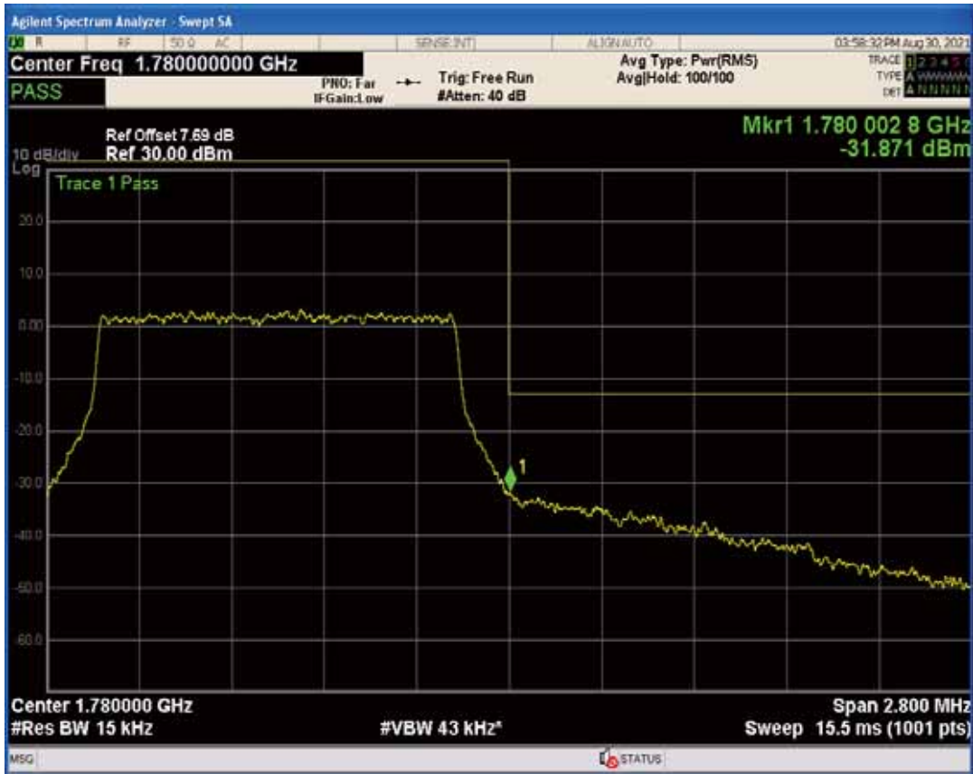
Band66 QPSK BW=3MHz Channel=131987 RB Size=1 Position=#Max
