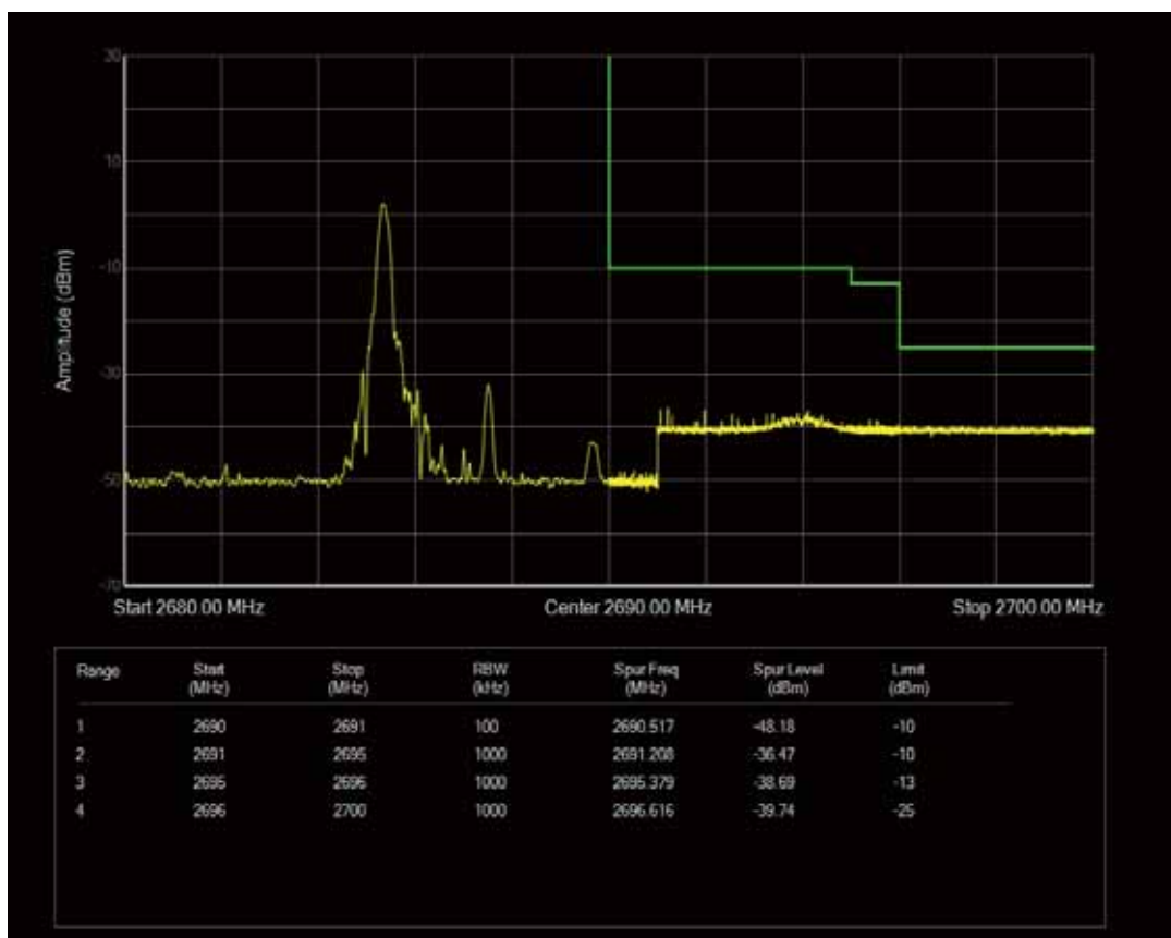
Band41 QAM16 BW=5MHz Channel=41565 RB Size=1 Position=#Max
