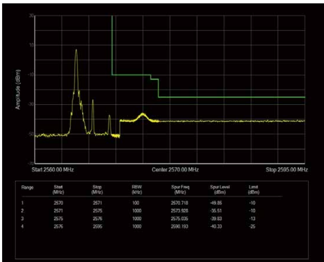
Band7 QAM16 BW=5MHz Channel=21425 RB Size=1 Position=#Max
