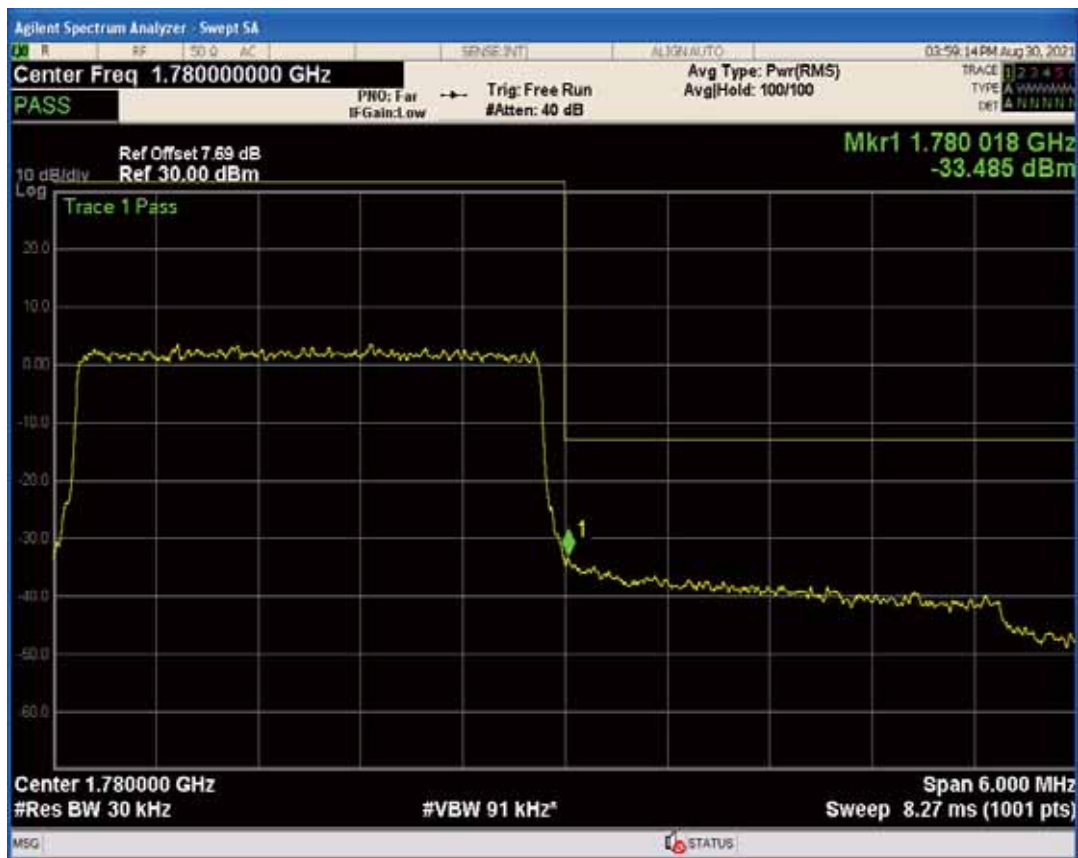
Band66 QAM16 BW=3MHz Channel=132657 RB Size=1 Position=#0
