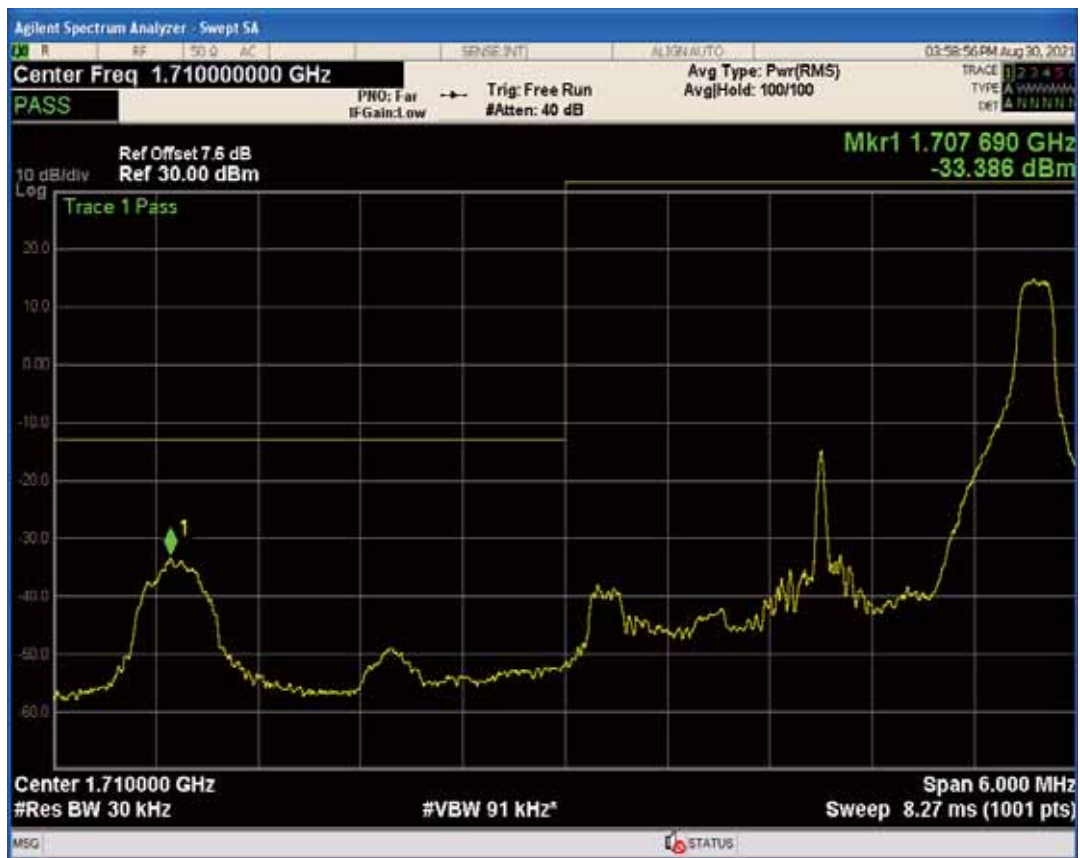
Band66 QPSK BW=3MHz Channel=132657 RB Size=1 Position=#0
