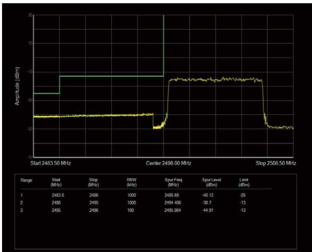
Band41 QPSK BW=10MHz Channel=41540 RB Size=1 Position=#Max
