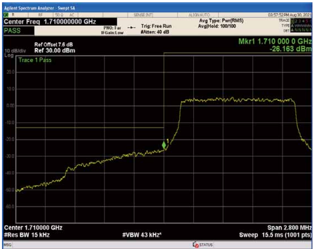
Band66 QAM16 BW=1.4MHz Channel=131979 RB Size=1 Position=#0
