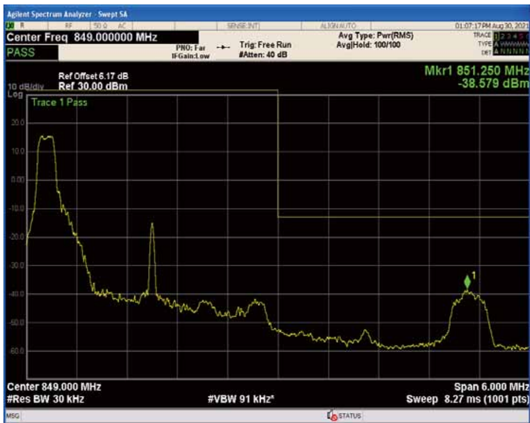
Band5 QAM16 BW=3MHz Channel=20415 RB Size=15 Position=#0
