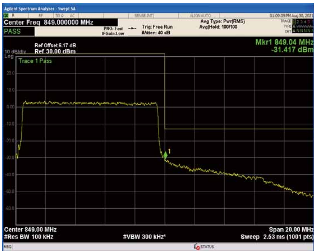
Band5 QAM16 BW=10MHz Channel=20600 RB Size=1 Position=#Max
