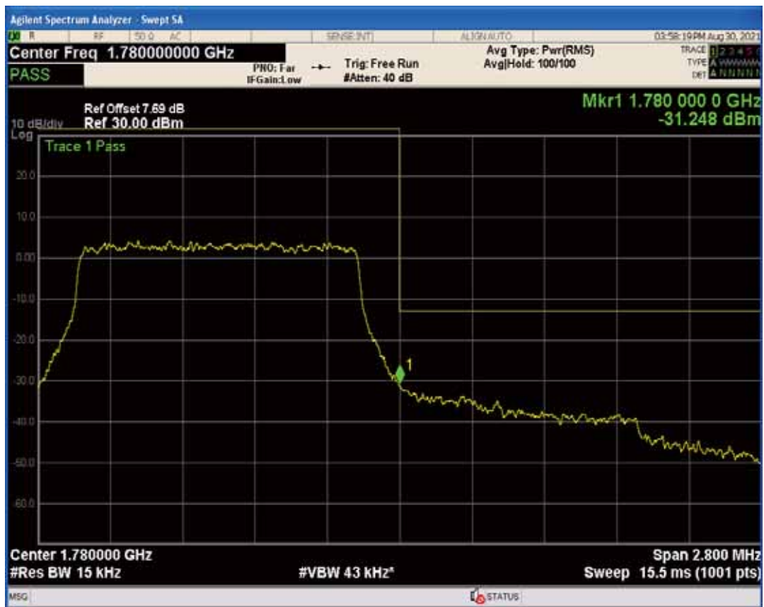
Band66 QAM16 BW=1.4MHz Channel=132665 RB Size=1 Position=#0
