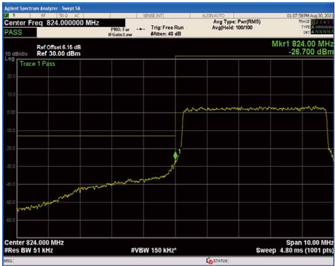
Band5 QAM16 BW=5MHz Channel=20425 RB Size=1 Position=#Max
