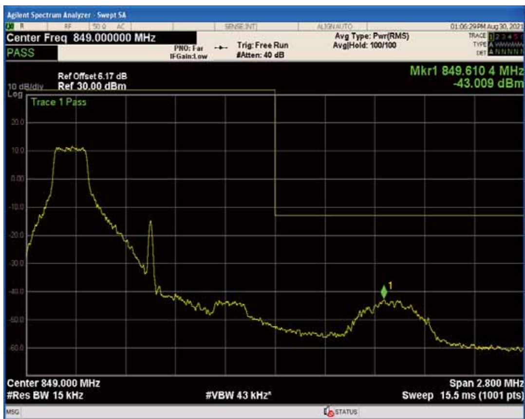
Band5 QAM16 BW=1.4MHz Channel=20643 RB Size=1 Position=#Max
