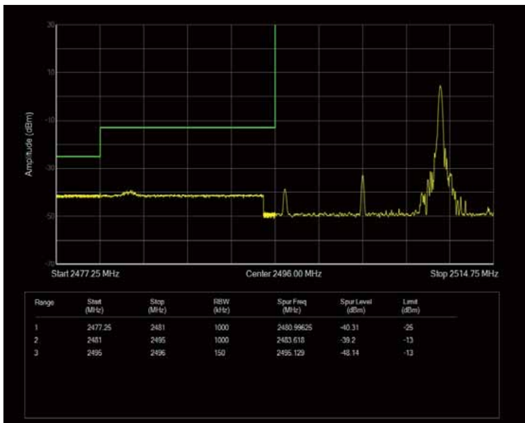
Band41 QPSK BW=15MHz Channel=39725 RB Size=1 Position=#0
