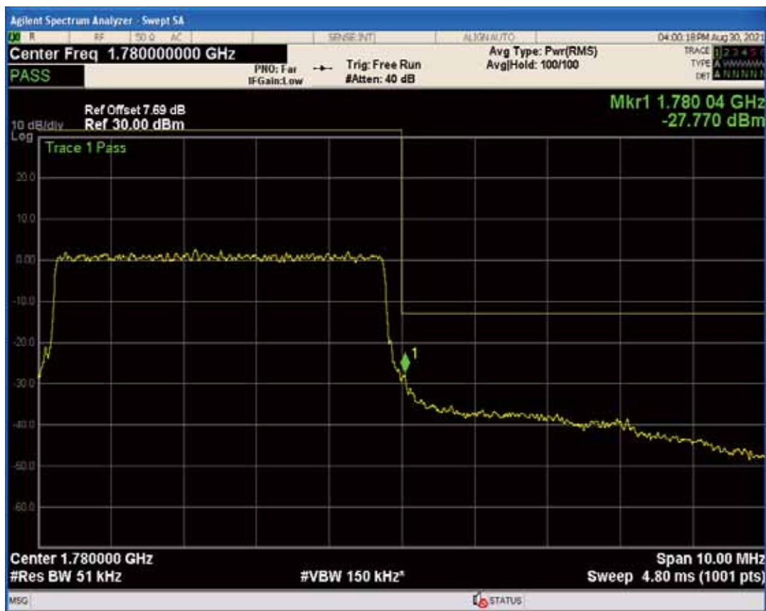
Band66 QPSK BW=10MHz Channel=132022 RB Size=1 Position=#Max
