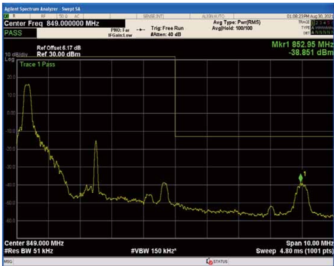
Band5 QAM16 BW=5MHz Channel=20625 RB Size=25 Position=#0
