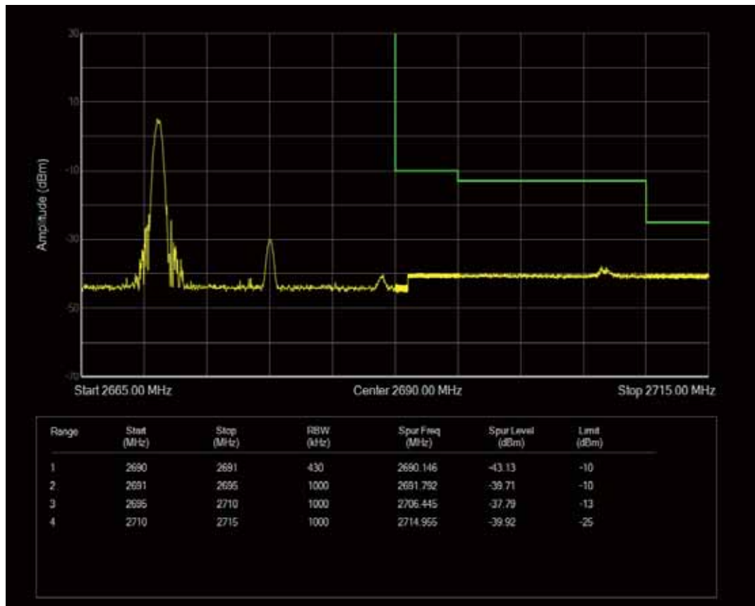
Band41 QAM16 BW=20MHz Channel=41490 RB Size=100 Position=#0
