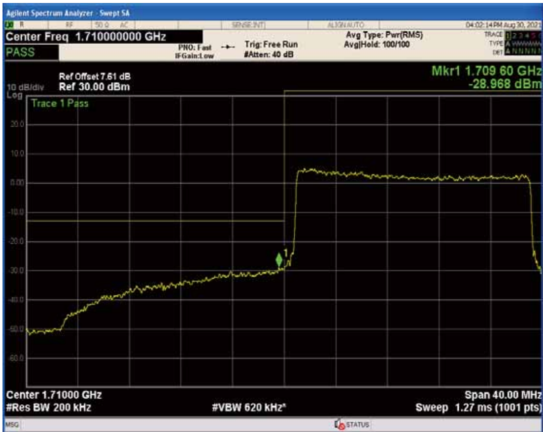
Band66 QAM16 BW=20MHz Channel=132072 RB Size=1 Position=#0
