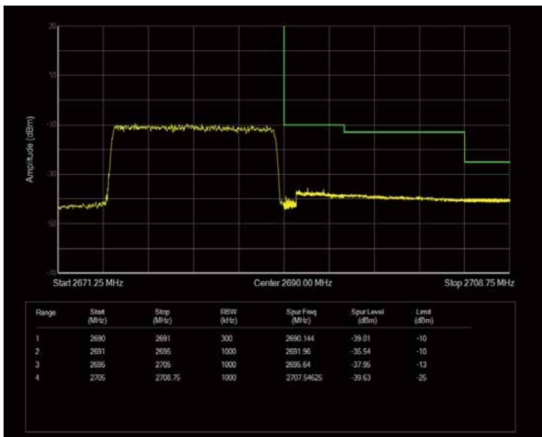
Band41 QAM16 BW=15MHz Channel=41515 RB Size=75 Position=#0
