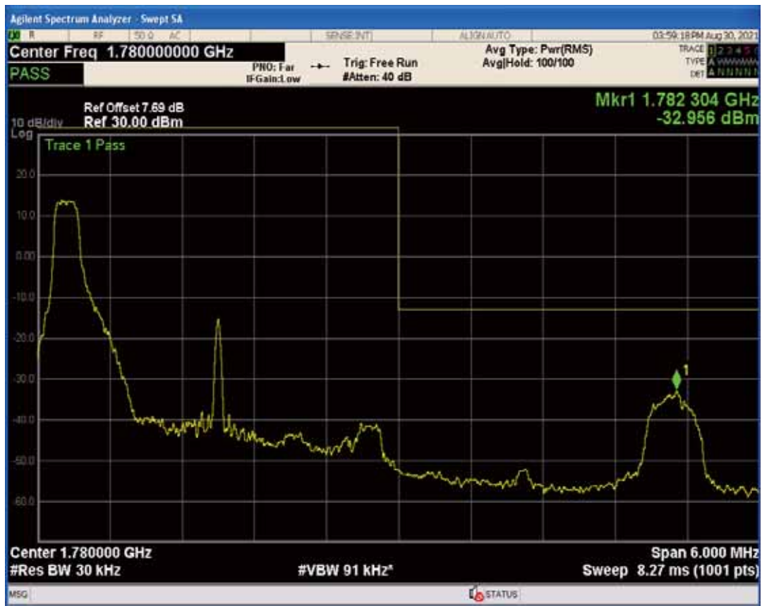
Band66 QAM16 BW=3MHz Channel=132657 RB Size=15 Position=#0
