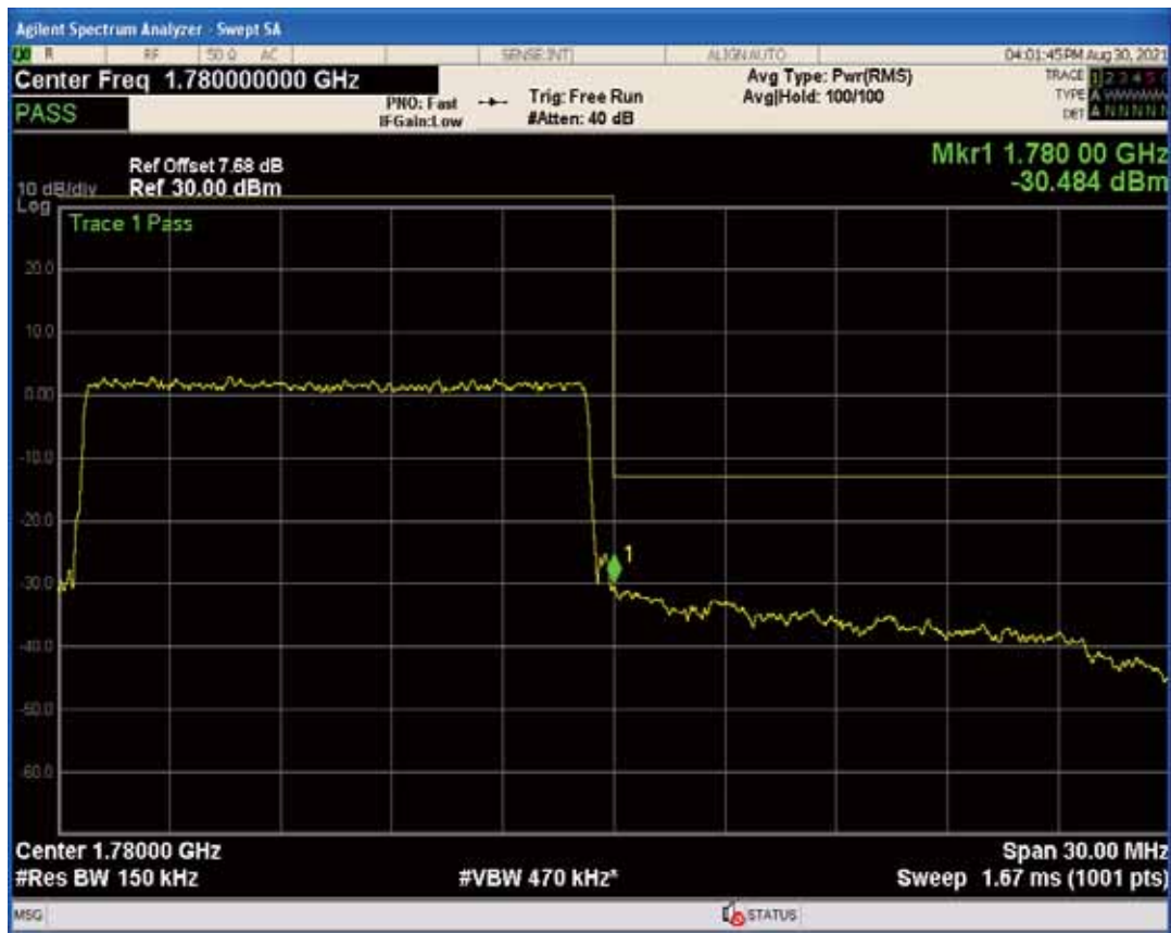
Band66 QPSK BW=15MHz Channel=132597 RB Size=1 Position=#Max
