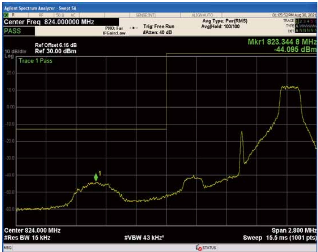
Band5 QAM16 BW=1.4MHz Channel=20407 RB Size=1 Position=#0
