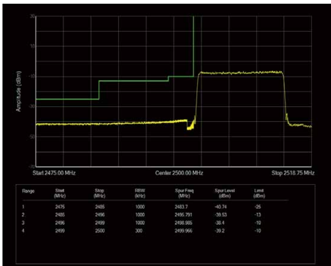
Band7 QAM16 BW=15MHz Channel=20825 RB Size=1 Position=#0
