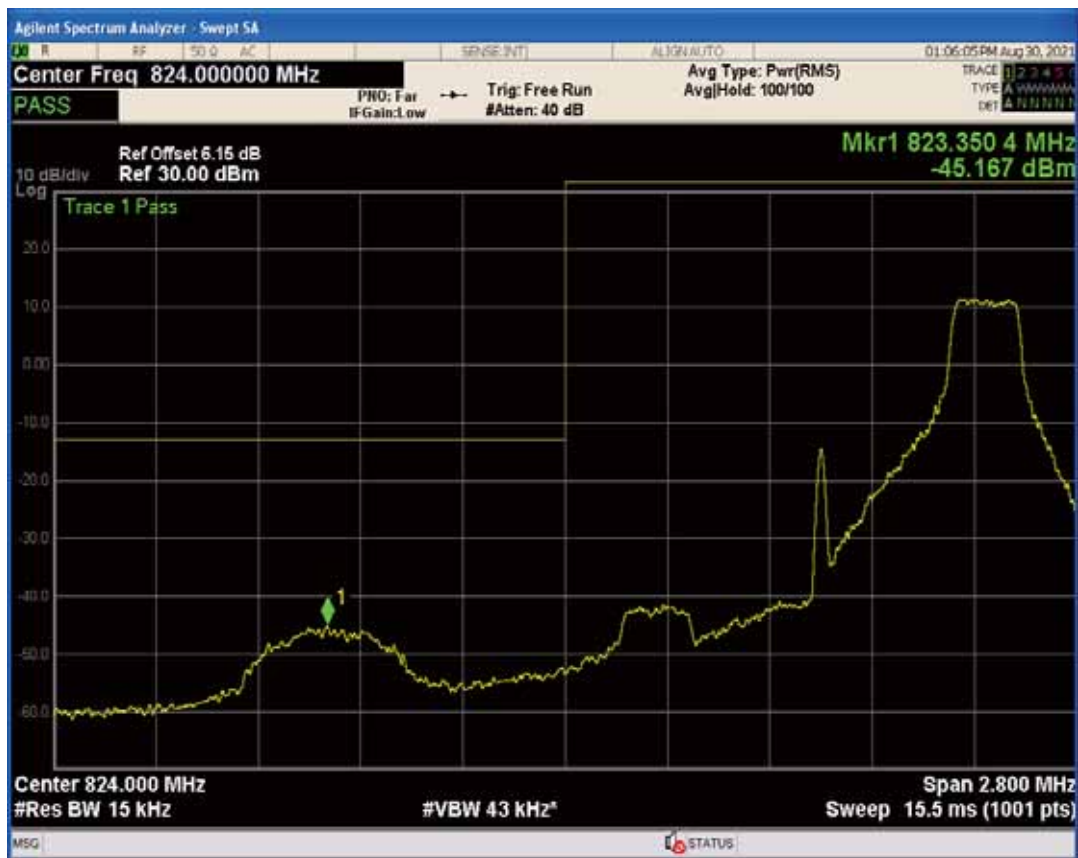
Band5 QAM16 BW=1.4MHz Channel=20407 RB Size=6 Position=#0
