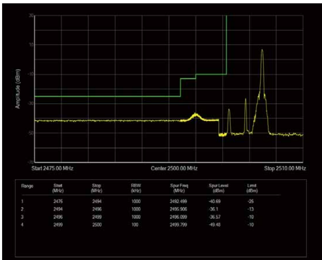
Band7 QPSK BW=5MHz Channel=20775 RB Size=25 Position=#0
