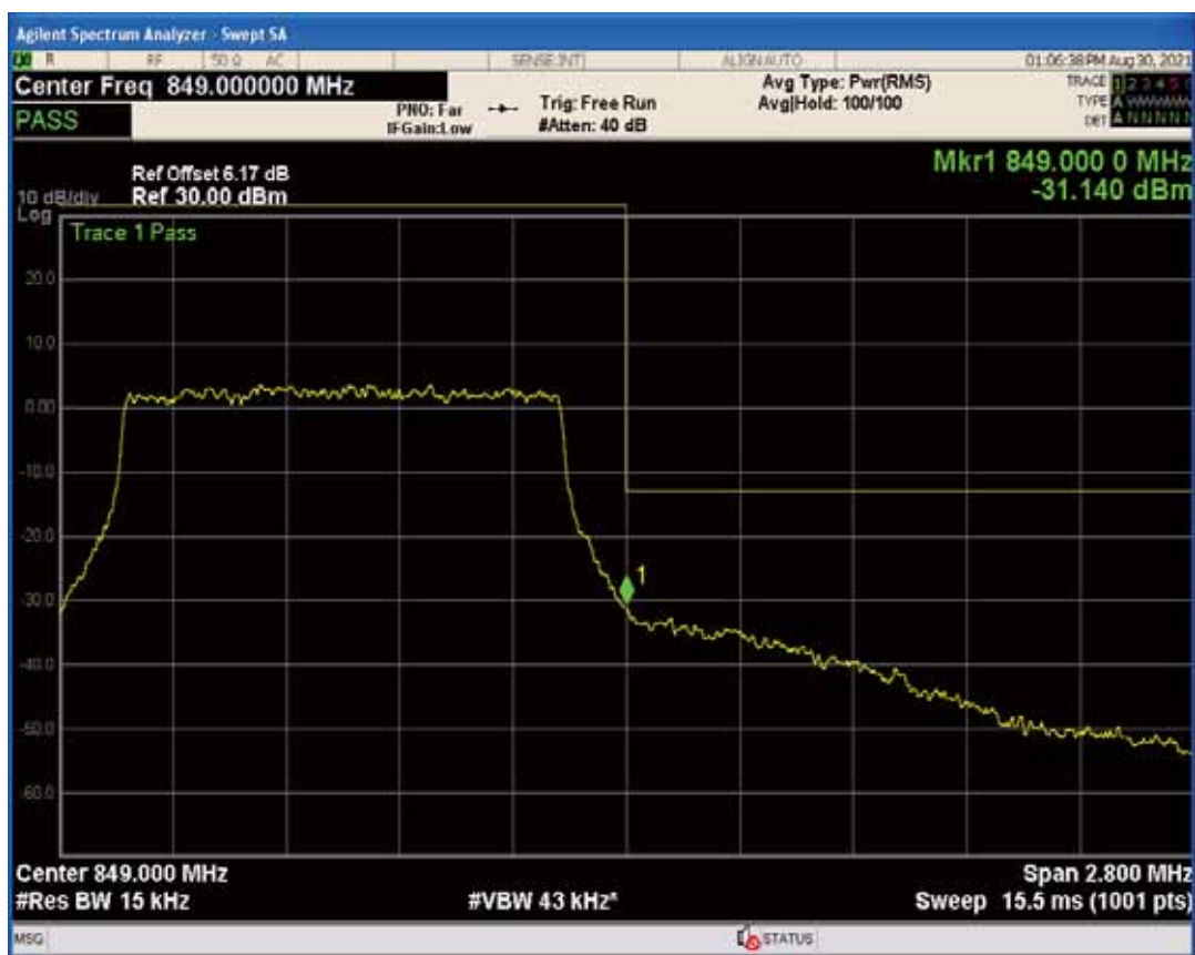
Band5 QPSK BW=3MHz Channel=20415 RB Size=1 Position=#0
