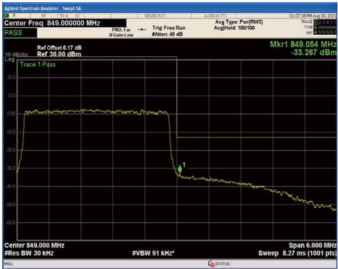
Band5 QPSK BW=5MHz Channel=20425 RB Size=1 Position=#0
