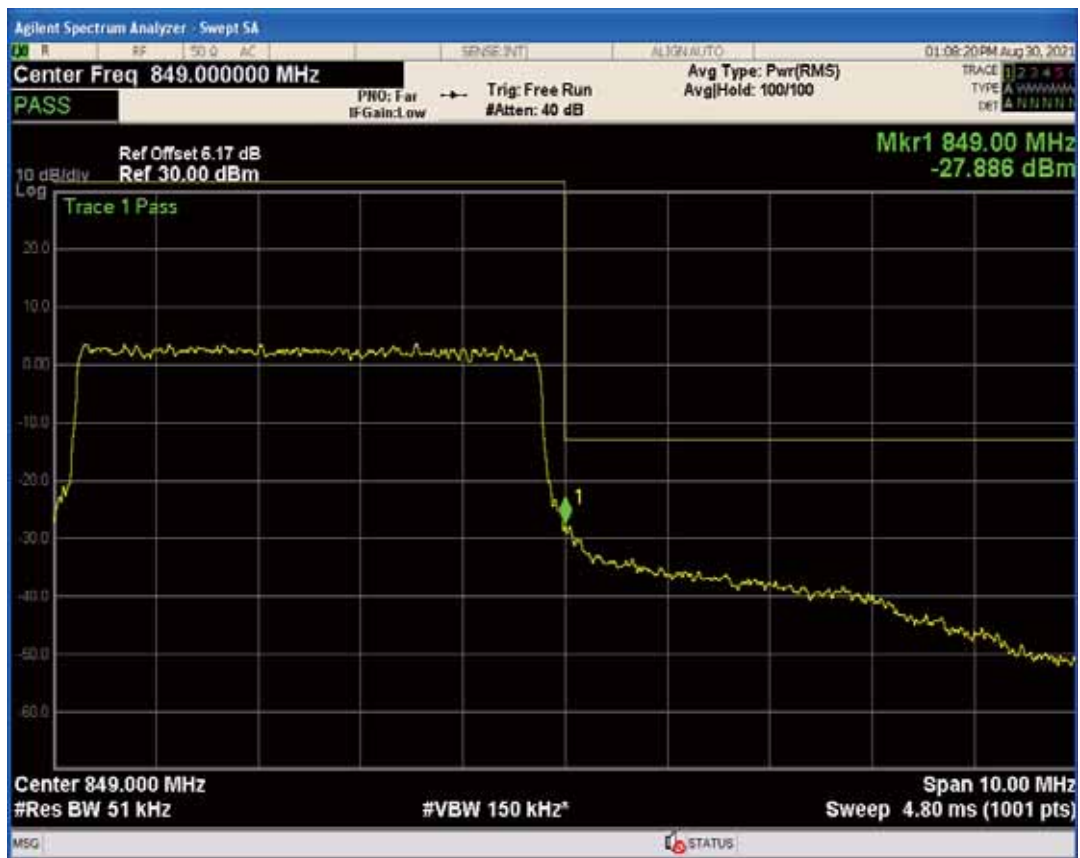
Band5 QAM16 BW=5MHz Channel=20625 RB Size=1 Position=#0
