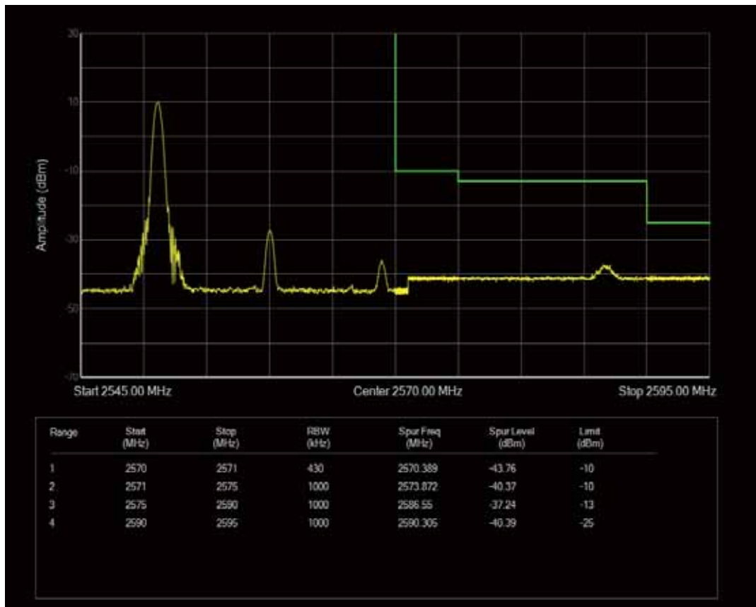
Band7 QAM16 BW=20MHz Channel=20850 RB Size=100 Position=#0
