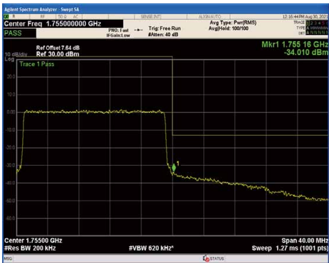
Band41 QPSK BW=5MHz Channel=39675 RB Size=1 Position=#0
