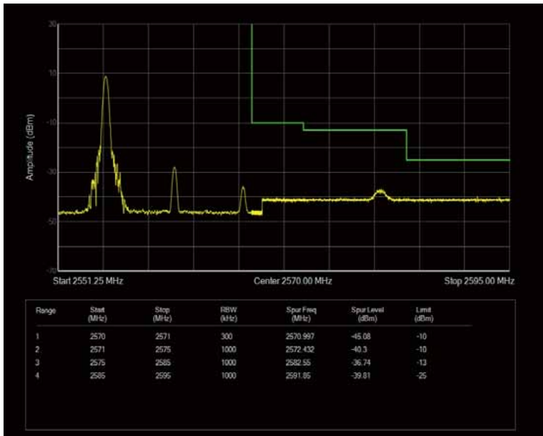
Band7 QAM16 BW=15MHz Channel=21375 RB Size=1 Position=#Max
