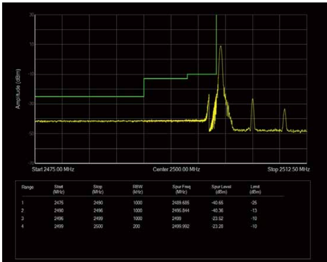
Band7 QPSK BW=10MHz Channel=20800 RB Size=50 Position=#0
