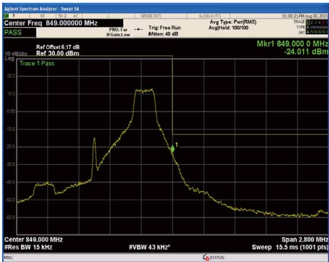
Band5 QPSK BW=1.4MHz Channel=20643 RB Size=6 Position=#0
