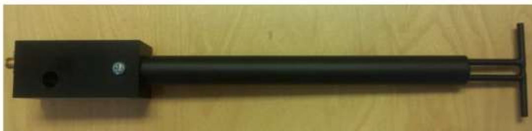
Figure 1 – MVG COMOSAR Validation Dipole
