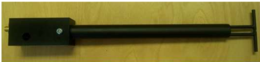
Figure 1 – MVG COMOSAR Validation Dipole
