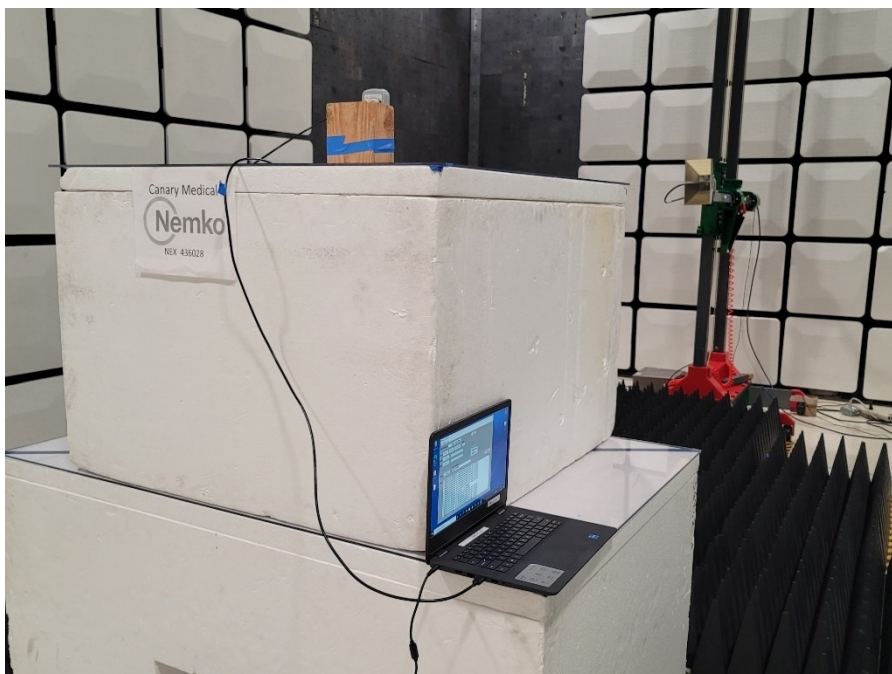
Figure 9- EIRP Measurement setup, rear view.
