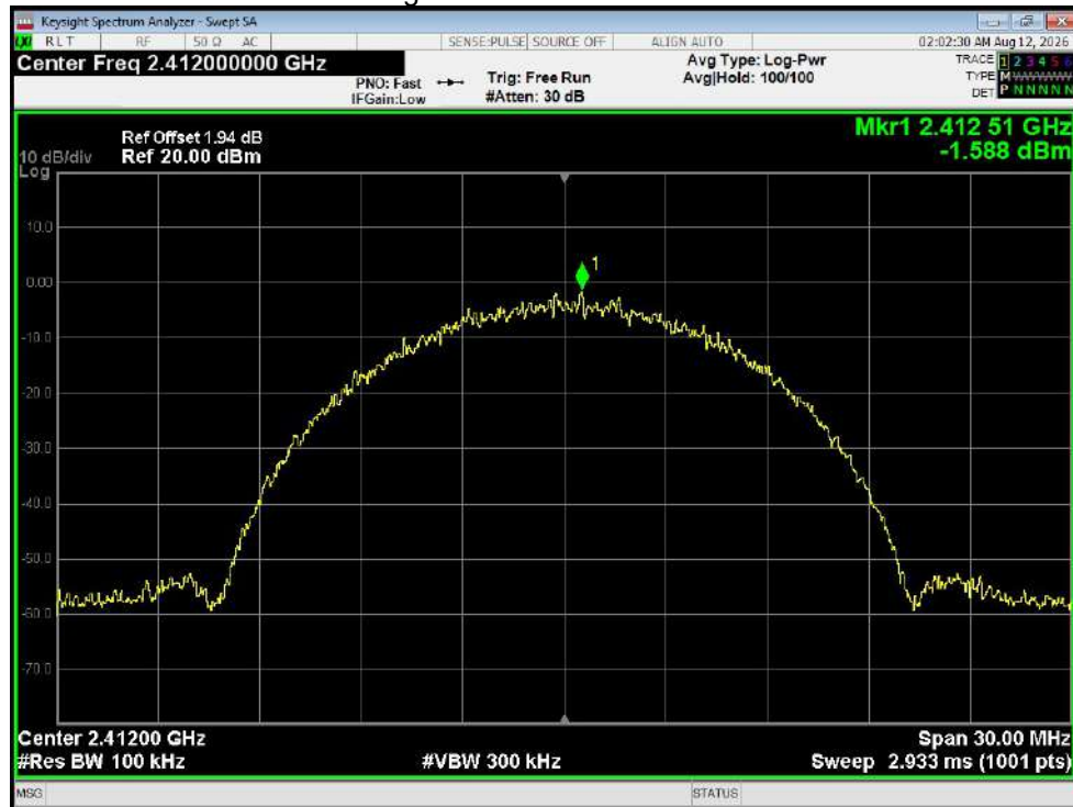
Band Edge NVNT b 2412MHz Ant1 Emission
