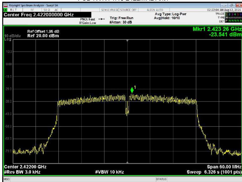
PSD NVNT n40 2422MHz Ant1
