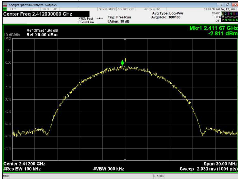
Tx. Spurious NVNT b 2412MHz Ant1 Emission
