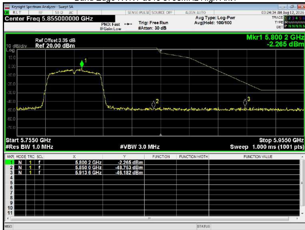
Band Edge NVNT ac40 5795MHz High Ant1
