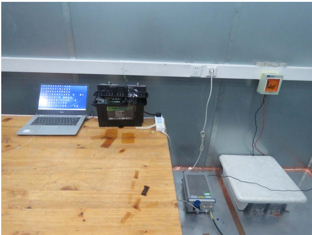
Picture 2 Conducted Emission Test Setup
