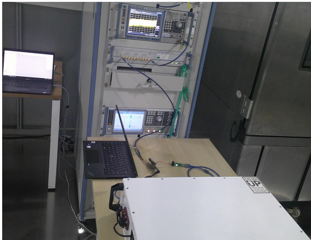
Photograph 1: Set-up photo for RF Conducted Test
