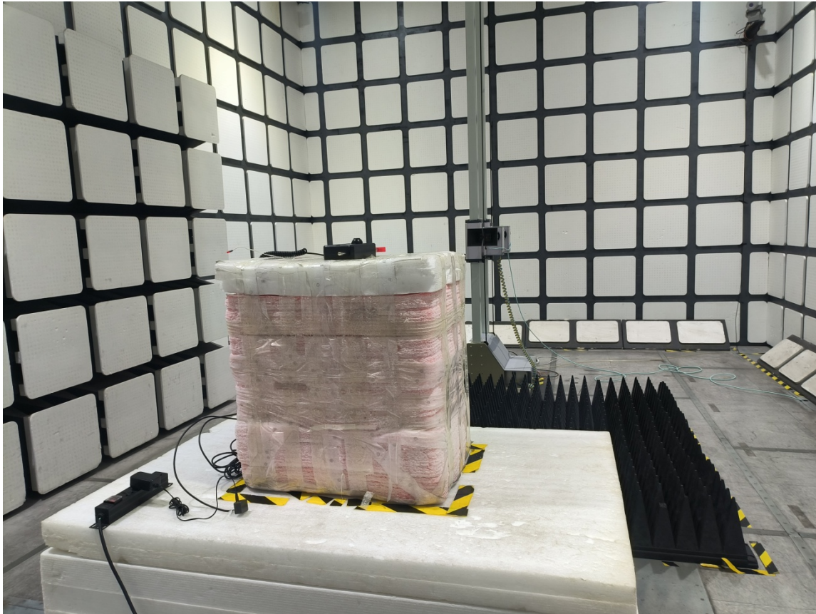
Radiated Emissions View (1-18 GHz)
