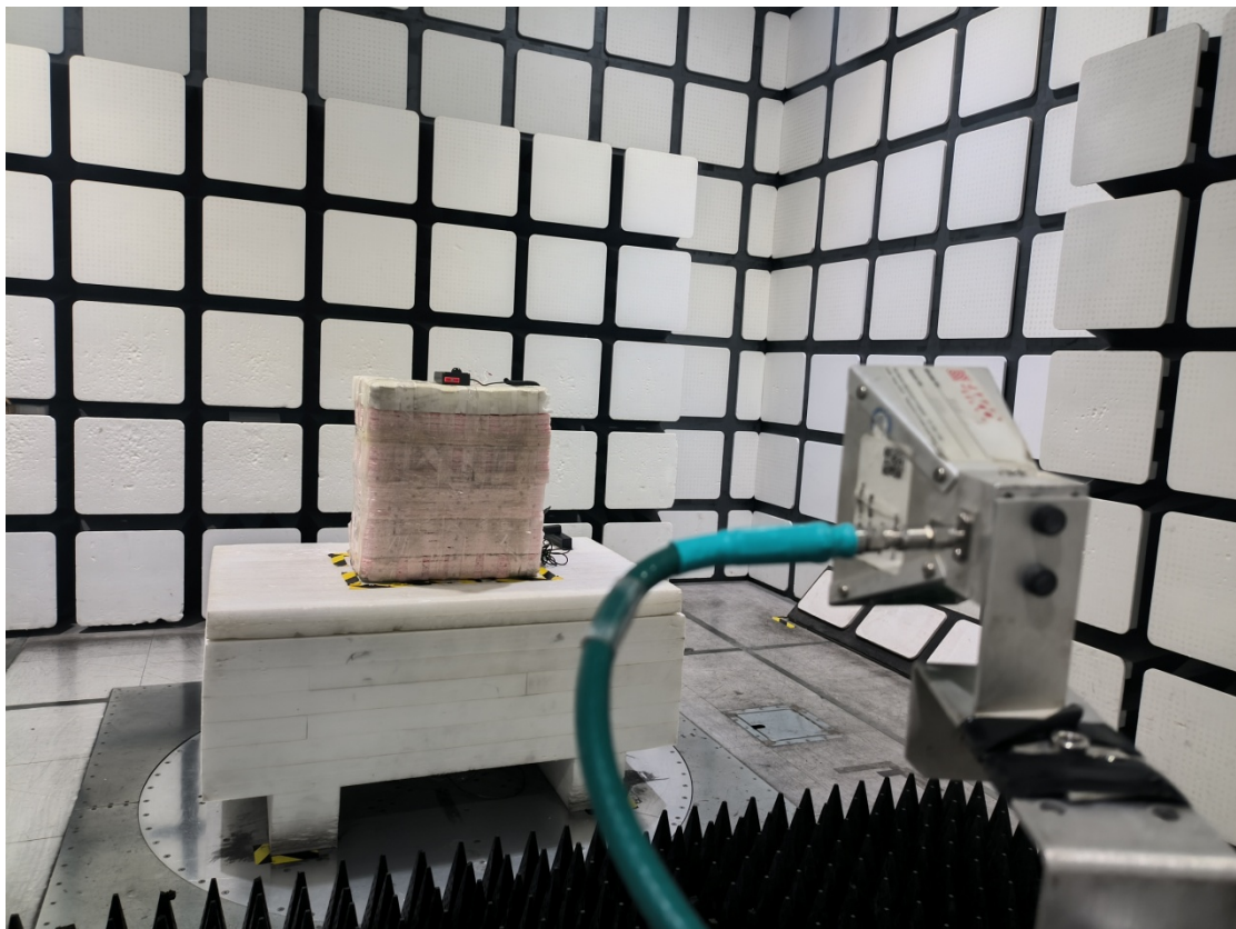
Radiated Emissions View (18-25 GHz)
