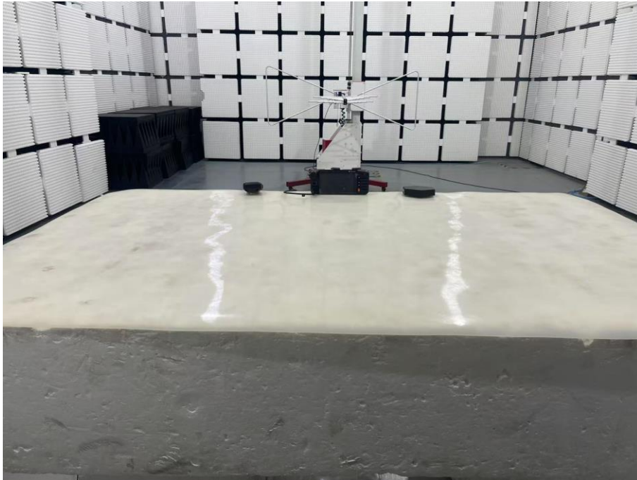
Set-up for Radiated Spurious Emission, Above 1GHz
