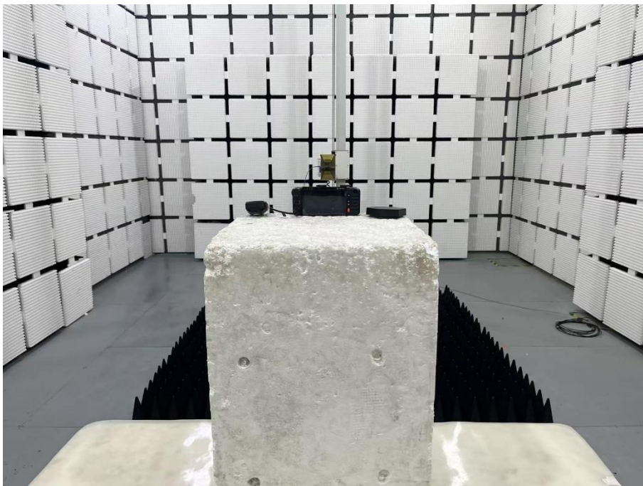
Set-up for Radiated Spurious Emission, Above 1GHz
