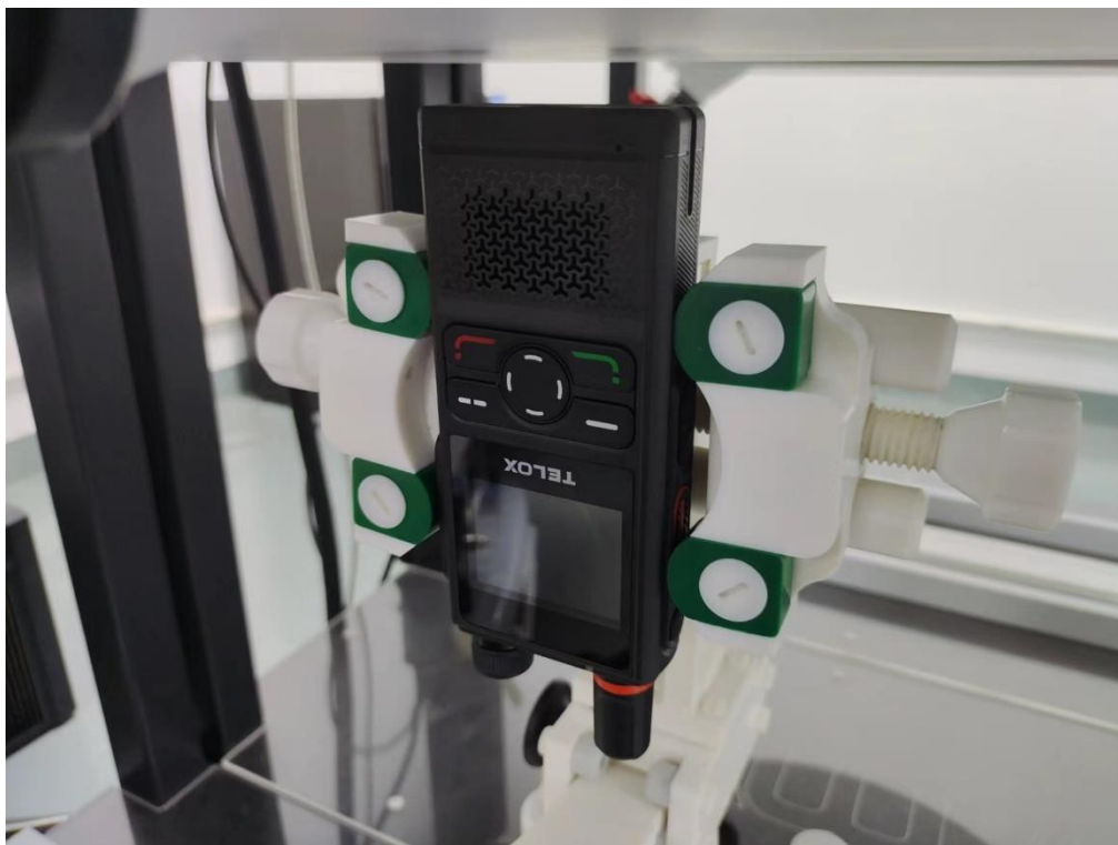
Body Bottom side (separation distance is 10mm)
