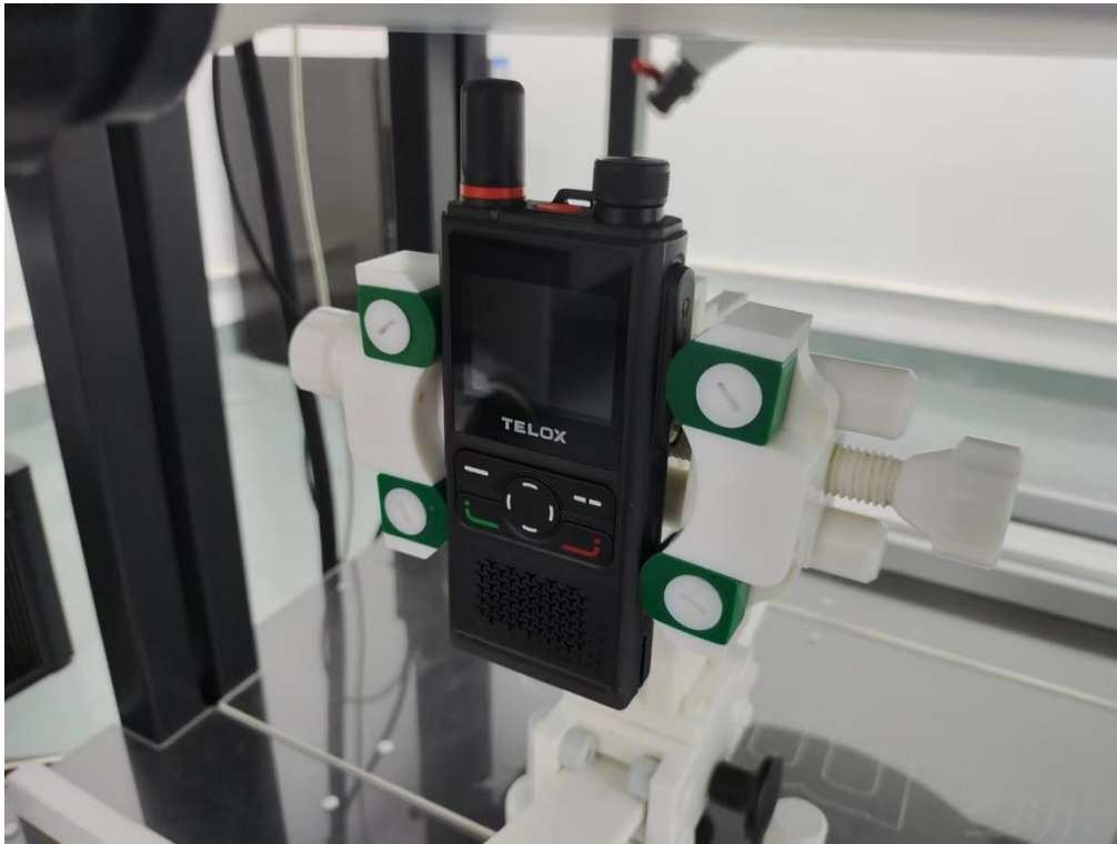
Body Top side (separation distance is 10mm)
