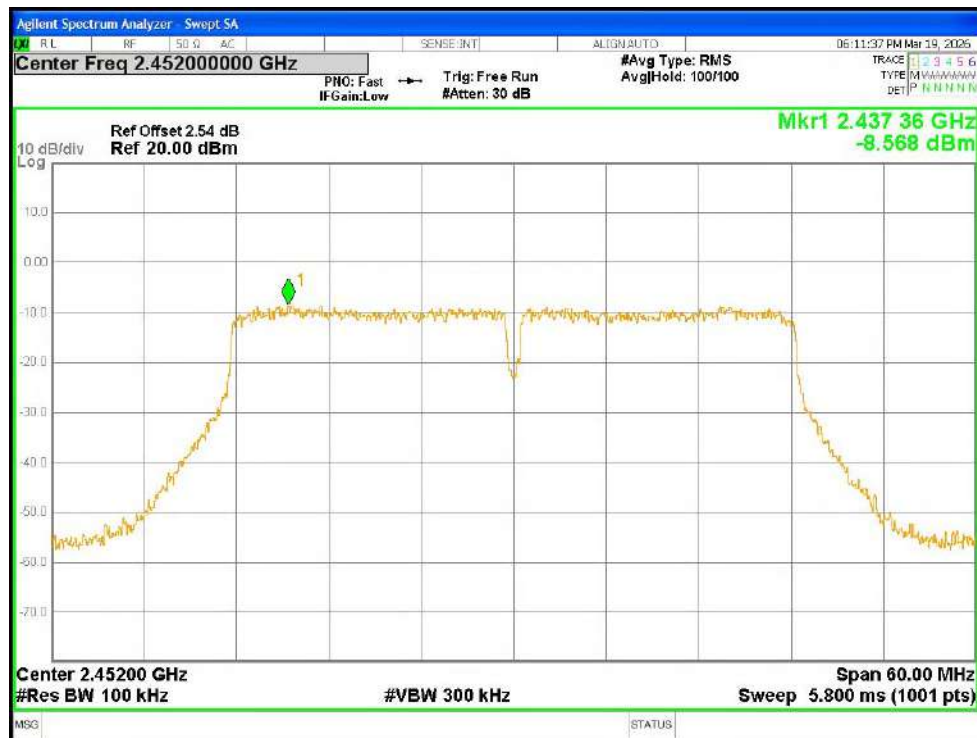
Tx. Spurious NVNT n40 2452MHz Ant1 Ref
