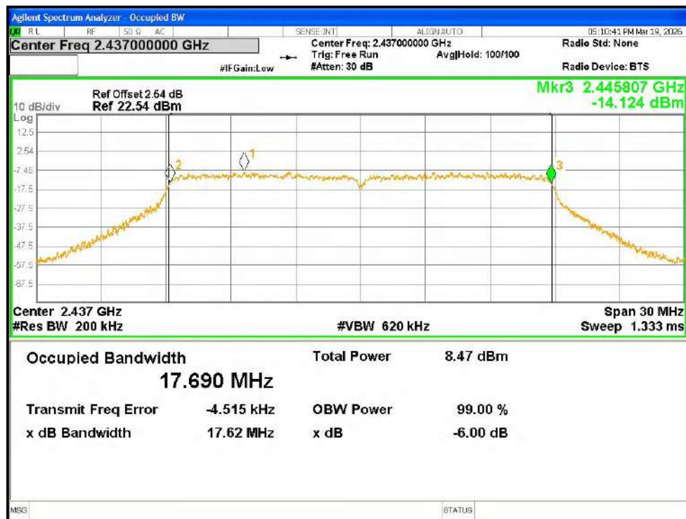
-6dB Bandwidth NVNT n20 2437MHz Ant1
