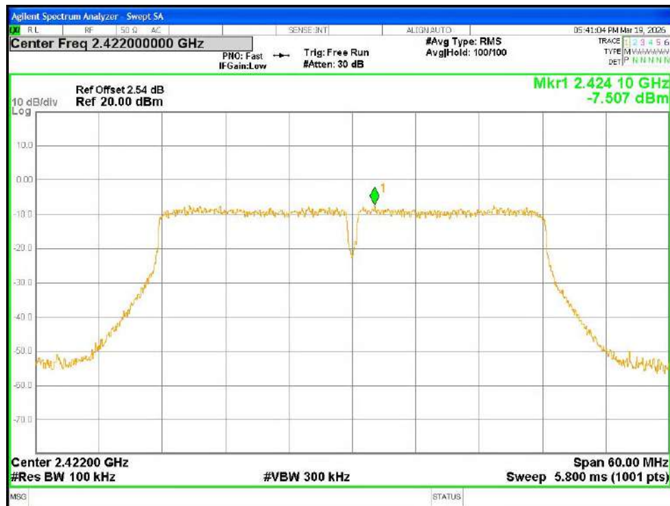
Tx. Spurious NVNT n40 2422MHz Ant1 Ref
