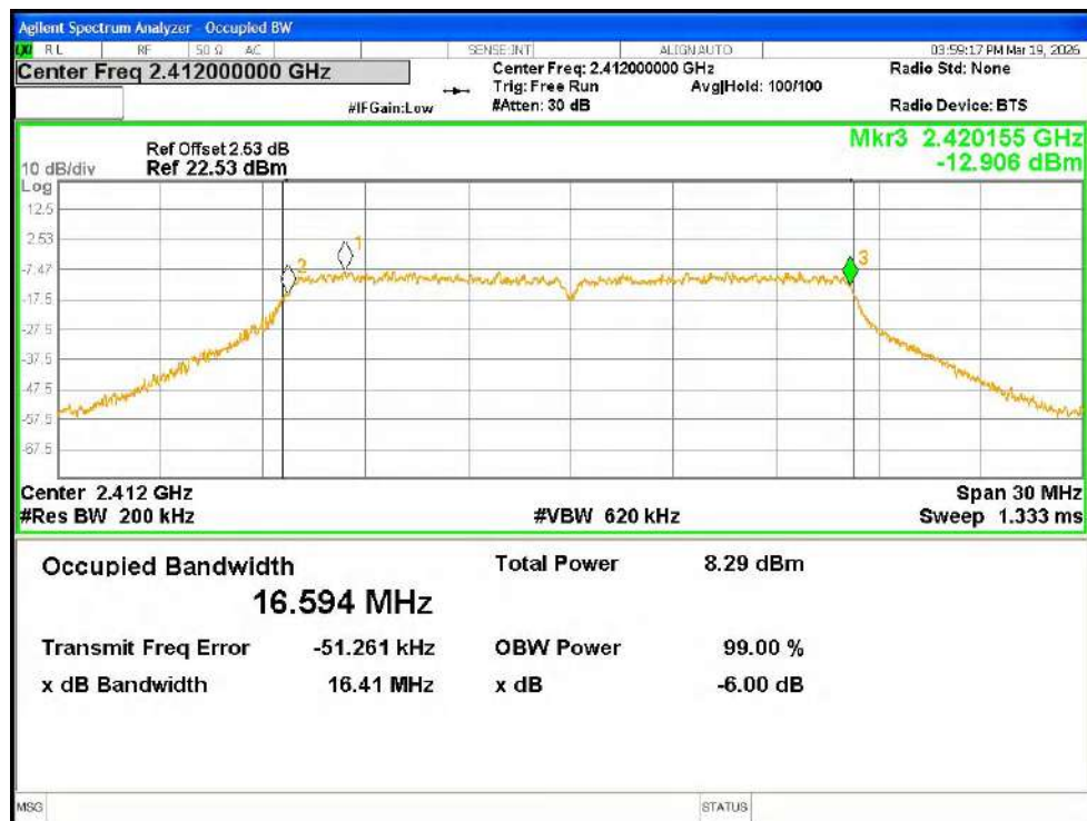
-6dB Bandwidth NVNT g 2412MHz Ant1
