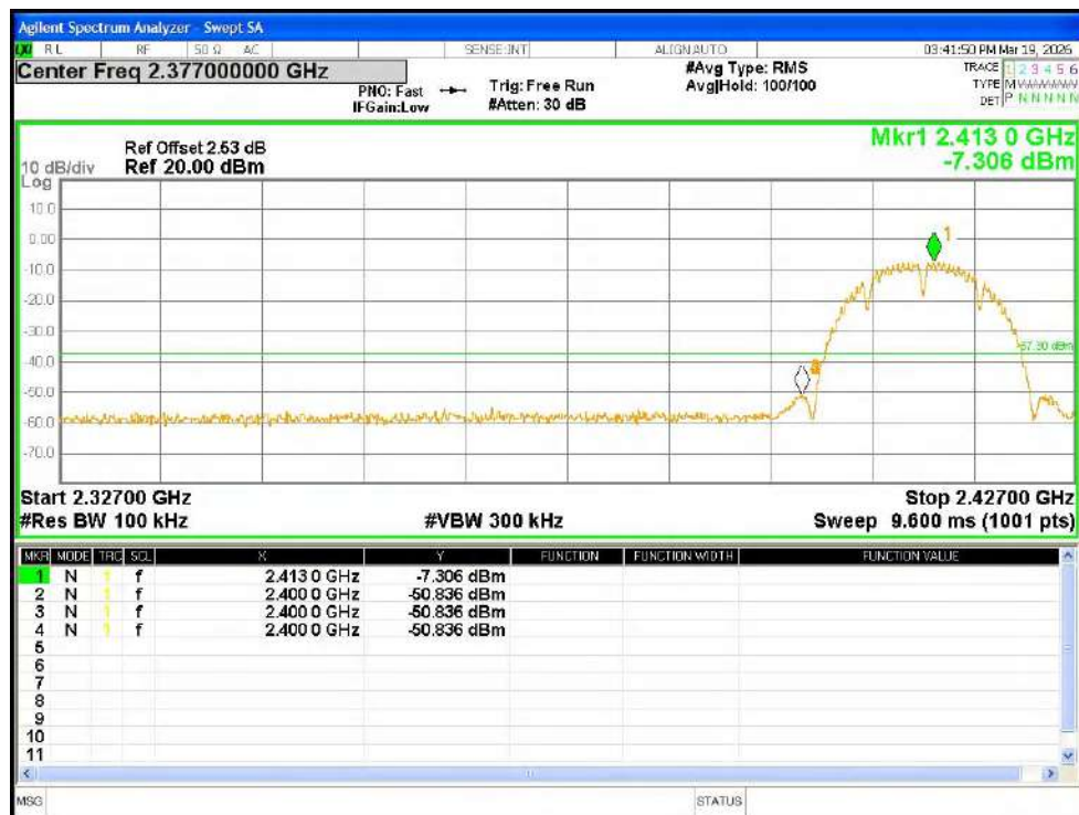
Band Edge NVNT b 2412MHz Ant1 Emission
