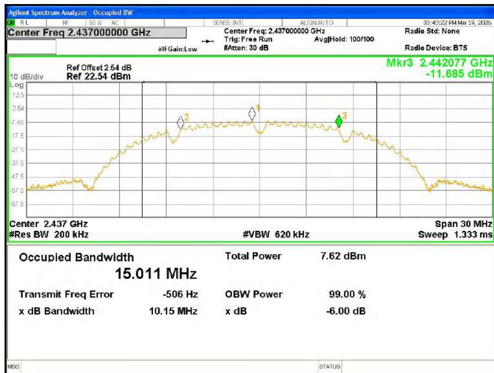
-6dB Bandwidth NVNT b 2437MHz Ant1
