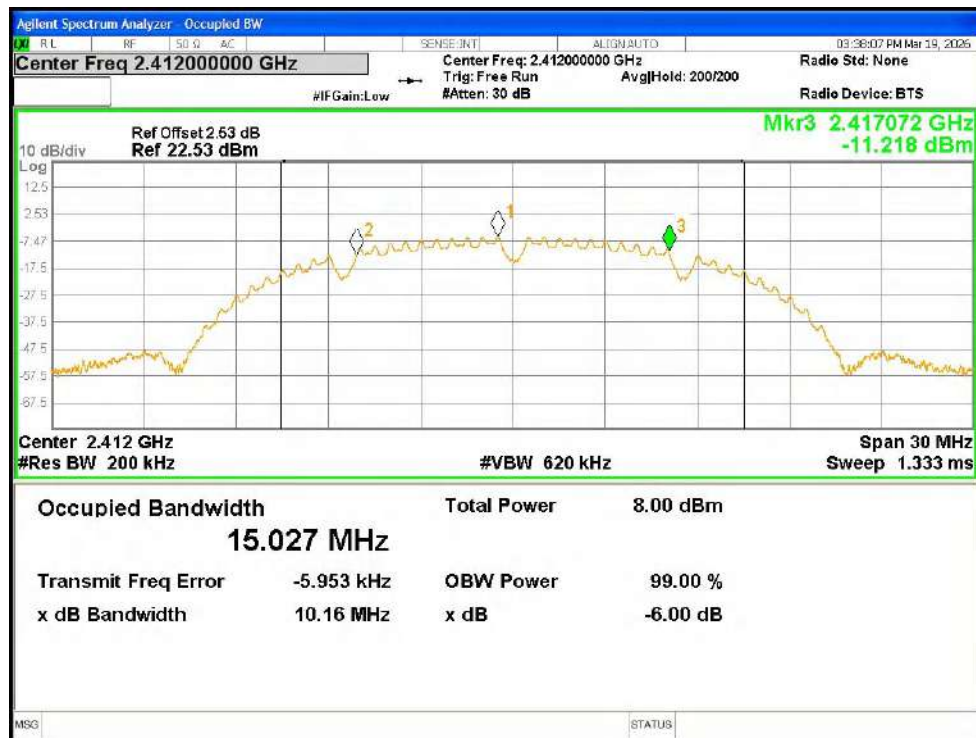
-6dB Bandwidth NVNT b 2412MHz Ant1
