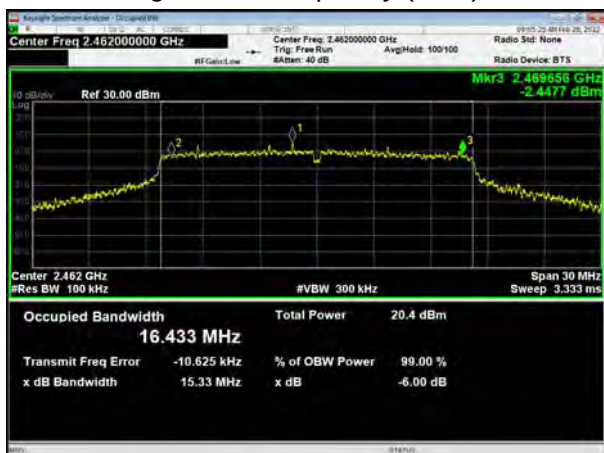
802.11g, Carrier frequency (MHz): 2462
