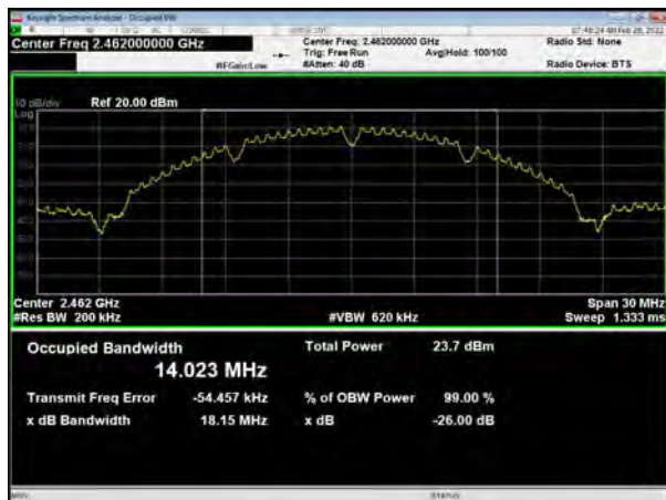
802.11b, Carrier frequency (MHz): 2462
