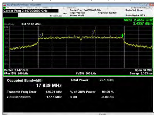
802.11n(HT20), Carrier frequency (MHz): 2457
