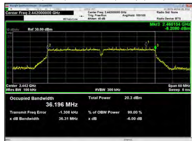
802.11n(HT40), Carrier frequency (MHz):2442
