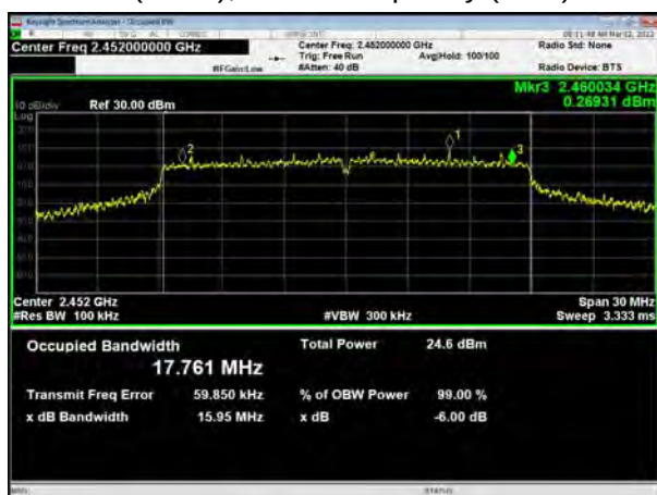
802.11n(HT20), Carrier frequency (MHz): 2452
