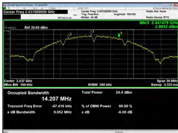
802.11b, Carrier frequency (MHz): 2462
