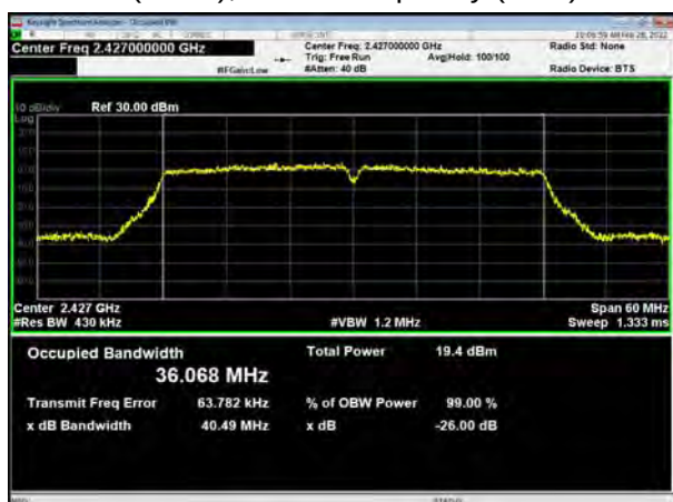
802.11n(HT40), Carrier frequency (MHz): 2427
