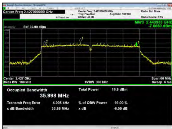
802.11n(HT40), Carrier frequency (MHz): 2427
