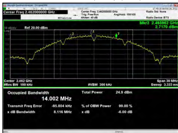
802.11b, Carrier frequency (MHz): 2462
