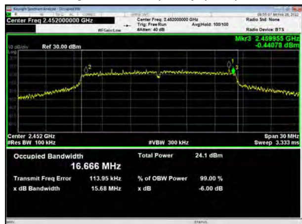
802.11g, Carrier frequency (MHz): 2452
