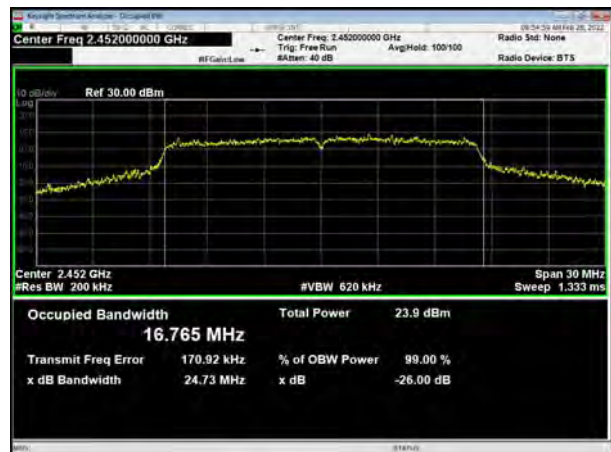
802.11g, Carrier frequency (MHz): 2452
