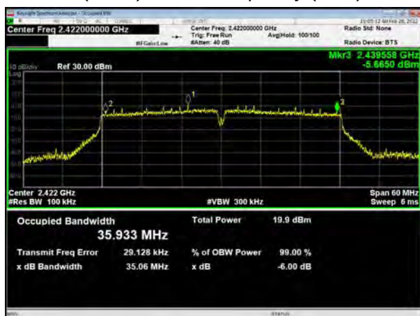
802.11n(HT40), Carrier frequency (MHz): 2427
