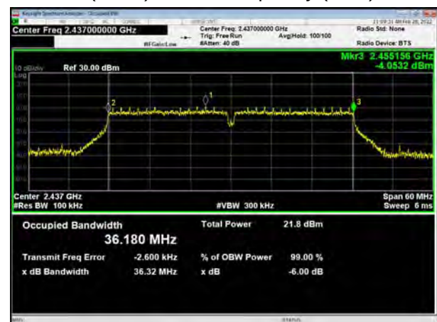
802.11n(HT40), Carrier frequency (MHz):2442
