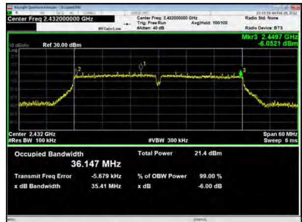
802.11n(HT40), Carrier frequency (MHz): 2437
