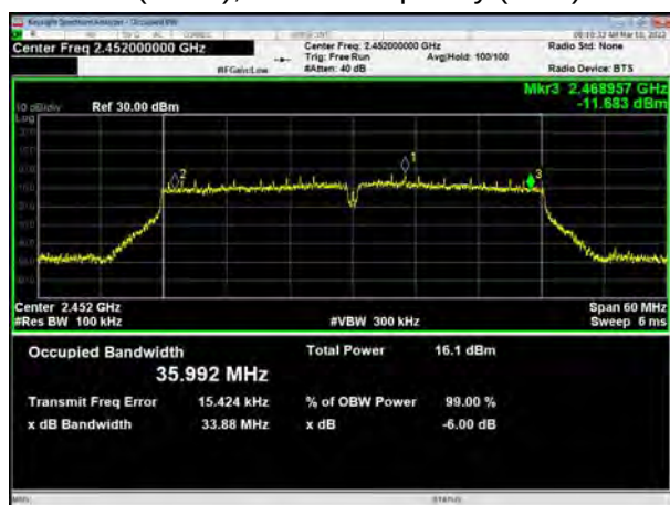
802.11n(HT40), Carrier frequency (MHz):2452
