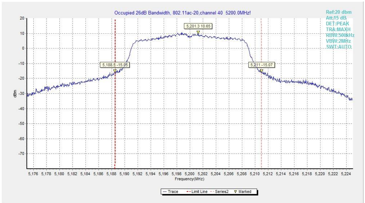
Fig.72 Occupied 26dB Bandwidth (802.11ac-VHT20, 5200MHz)
