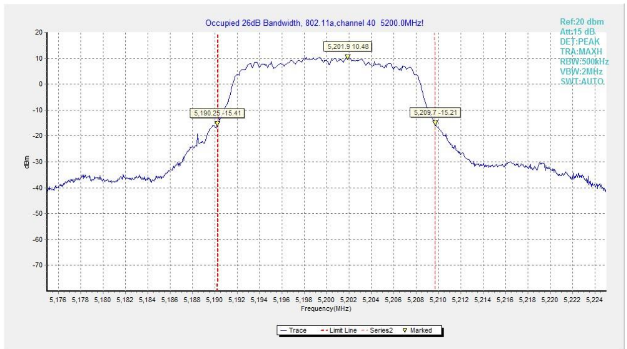
Fig.62 Occupied 26dB Bandwidth (802.11a, 5200MHz)
