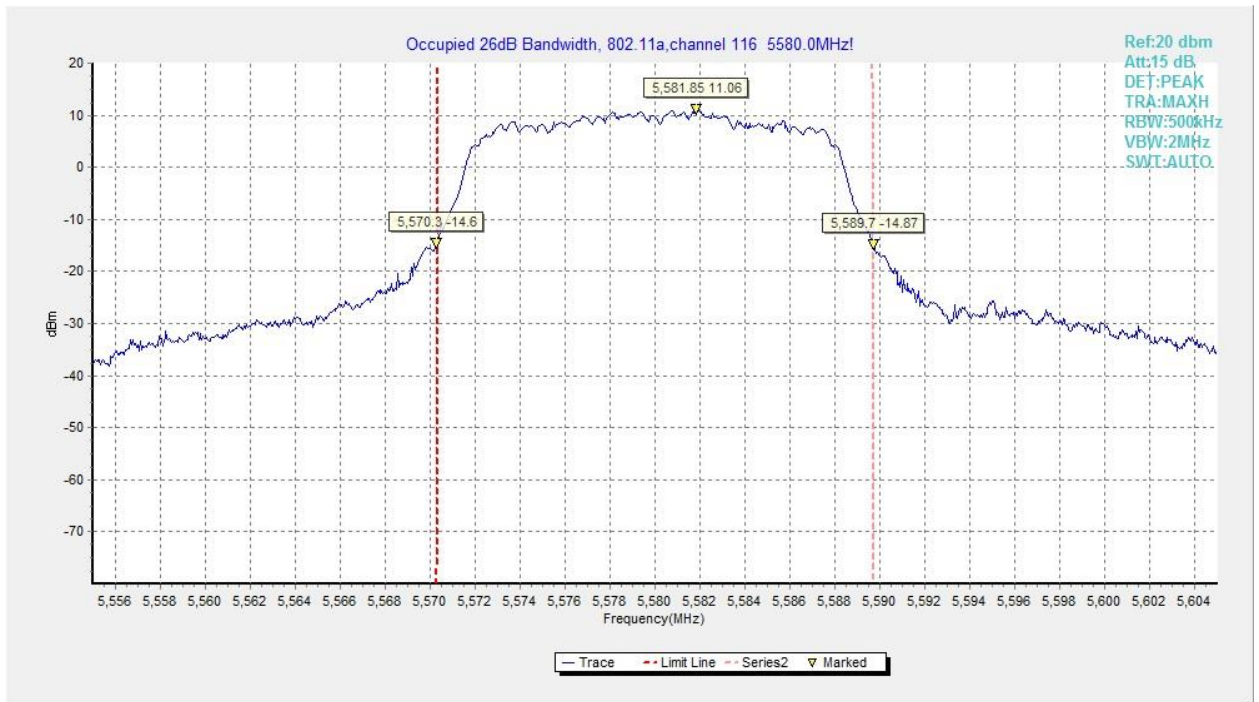
Fig.68 Occupied 26dB Bandwidth (802.11a, 5580MHz)
