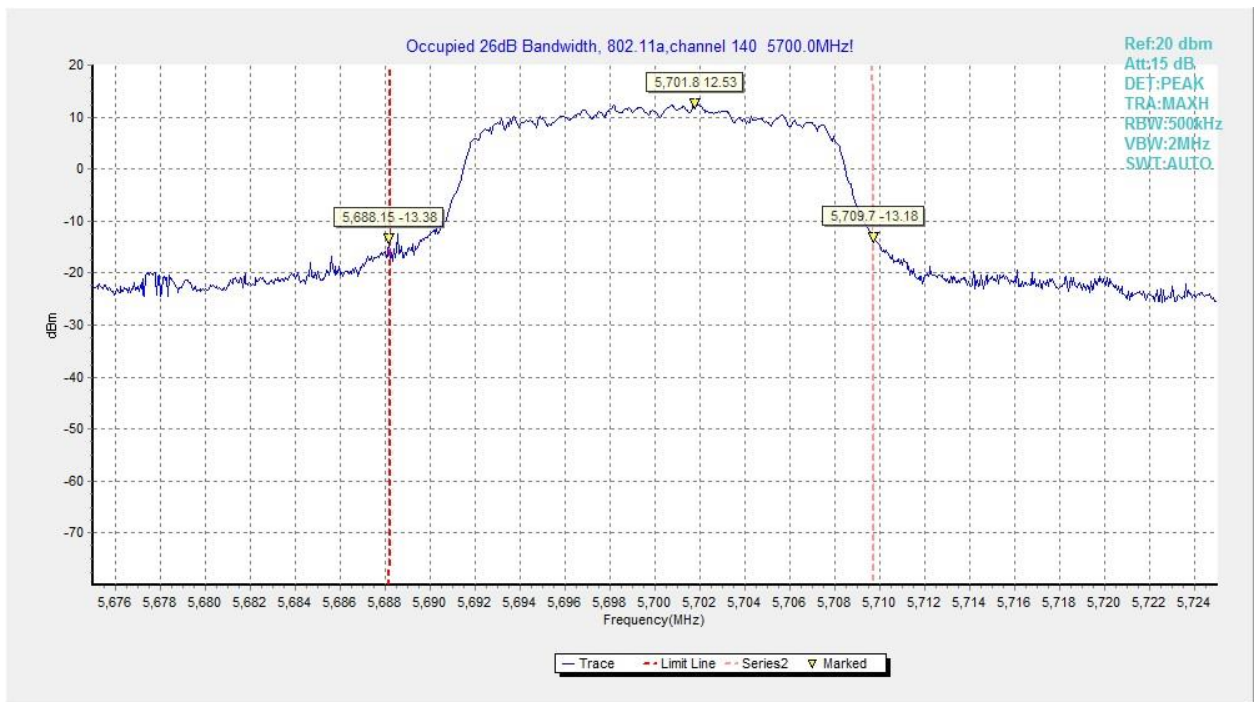
Fig.69 Occupied 26dB Bandwidth (802.11a, 5700MHz)
