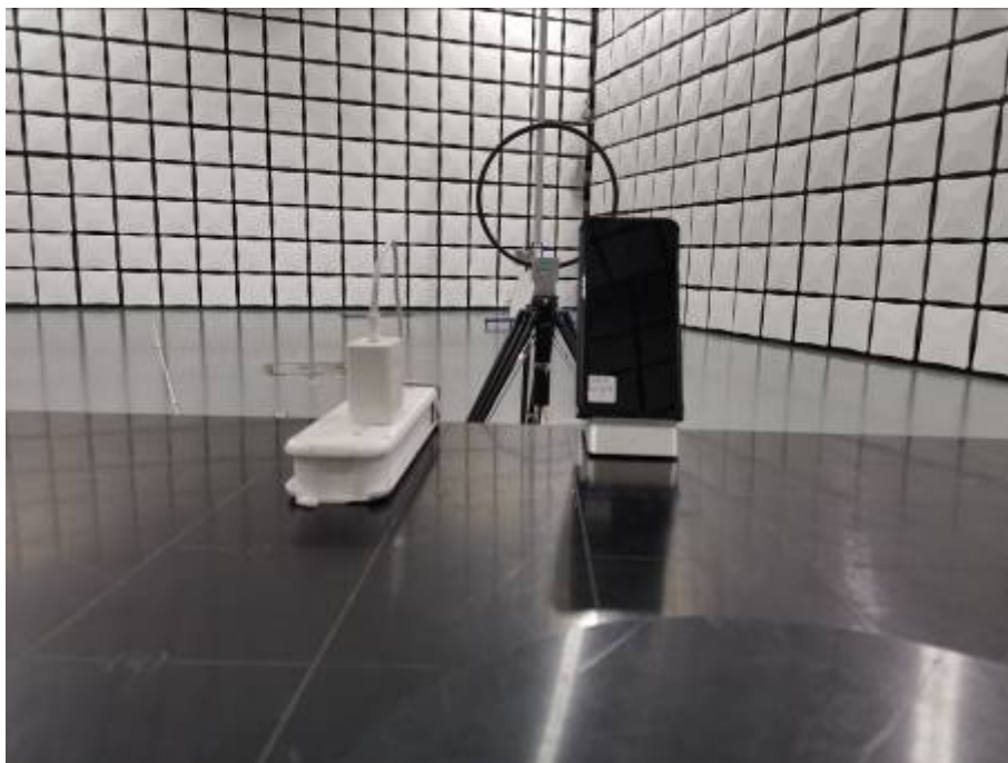
Radiated Emissions Test Setup (9KHz-30MHz)
