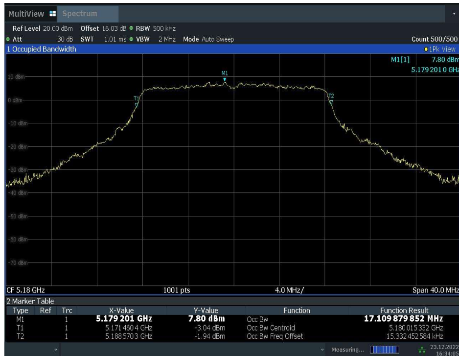
Fig.34 99% Occupied bandwidth (802.11a, 5180MHz)
