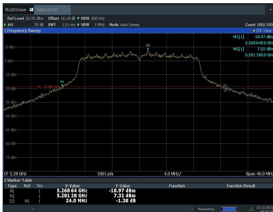
Fig.15 Occupied 26dB Bandwidth (802.11ac-VHT20, 5280MHz)
