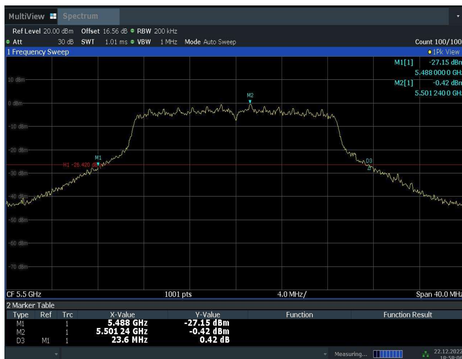
Fig.17 Occupied 26dB Bandwidth (802.11ac-VHT20, 5500MHz)
