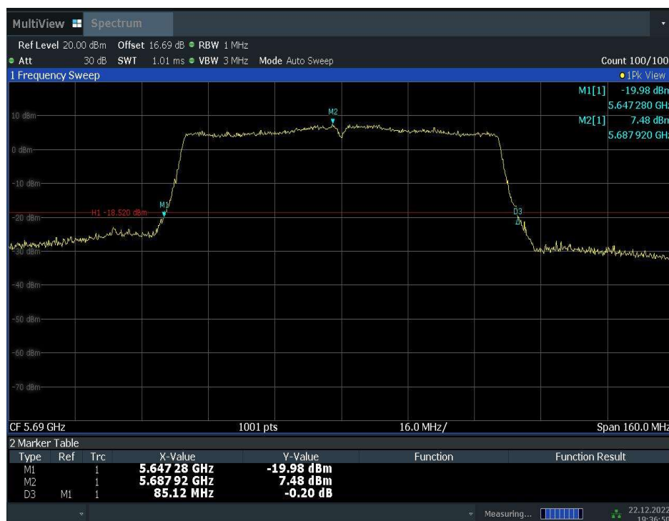
Fig.33 Occupied 26dB Bandwidth (802. 11ac-VHT80, 5690MHz)
