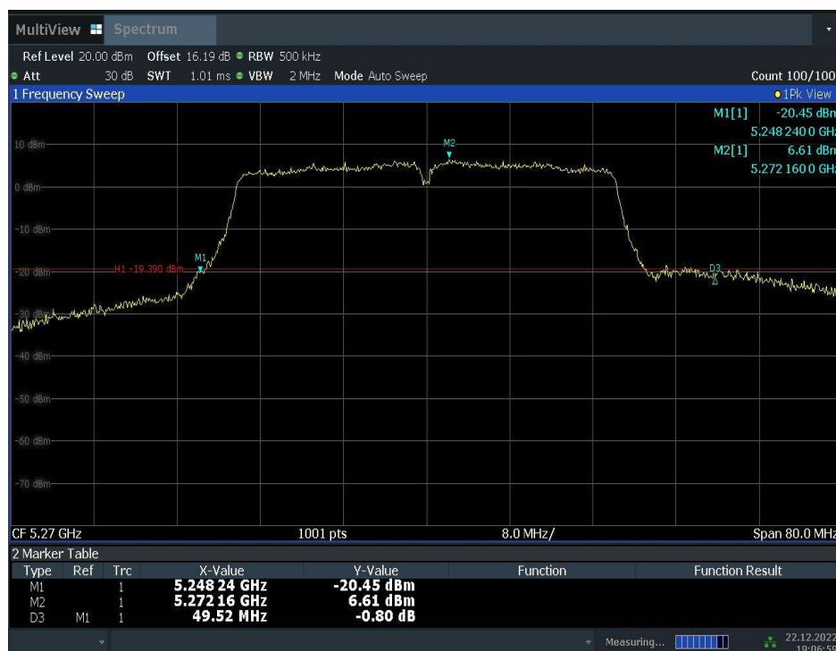
Fig.23 Occupied 26dB Bandwidth (802.11ac-VHT40, 5270MHz)
