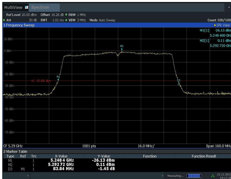
Fig.30 Occupied 26dB Bandwidth (802. 11ac-VHT80, 5290MHz)
