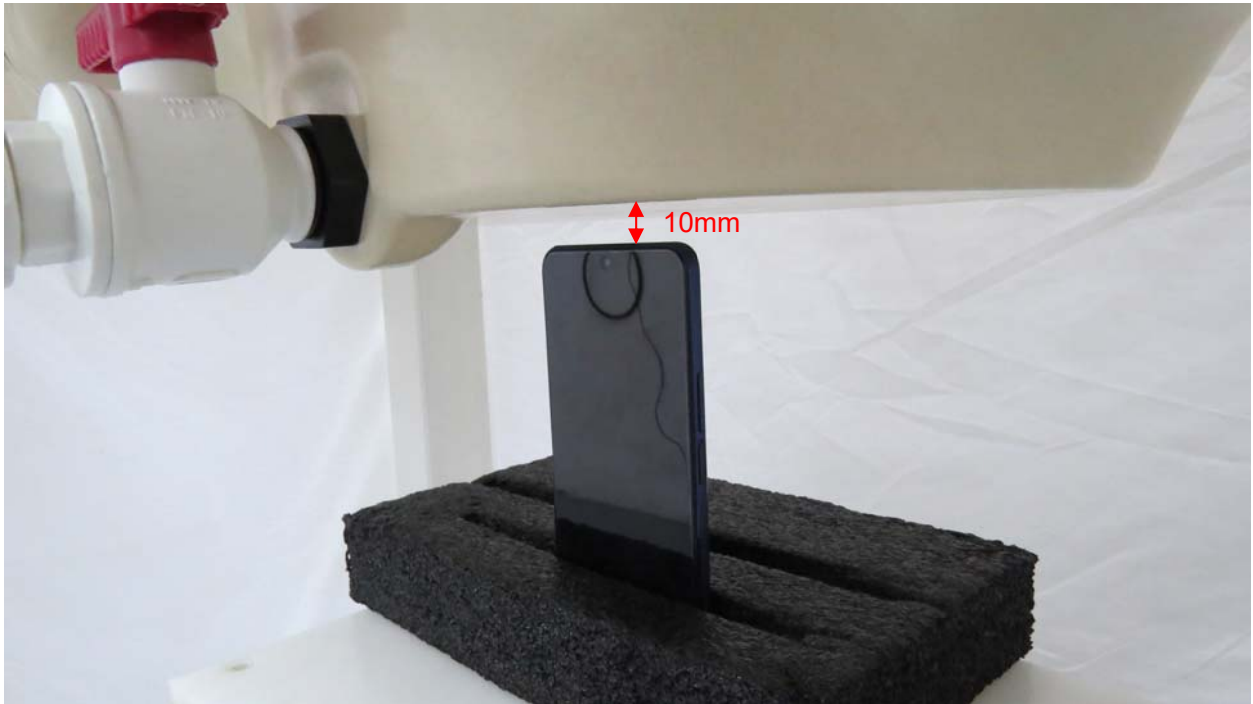
Picture 11: Top Side, the distance from handset to the bottom of the Phantom is 10mm
