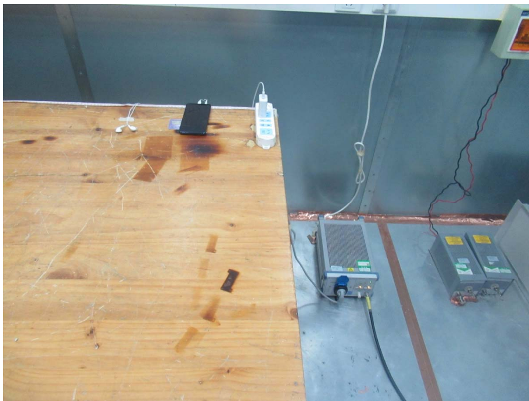
Picture 2 Conducted Emission Test Setup
