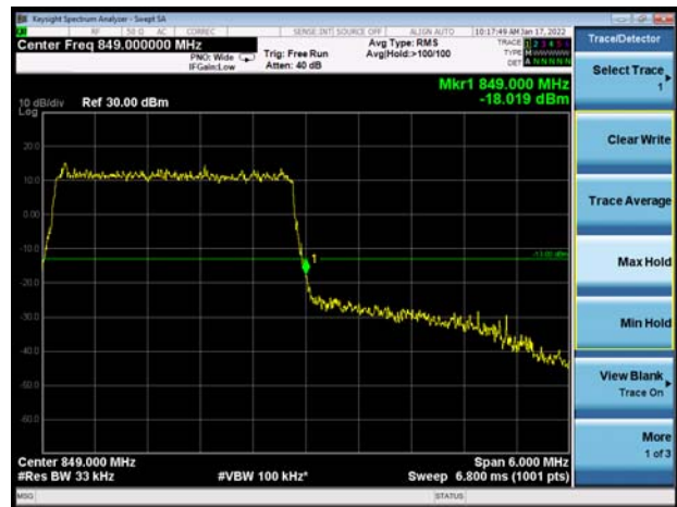
LTE Band 26 QPSK 5MHz CH-High 1RB
