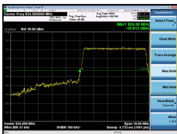
LTE Band 5 16QAM 10MHz CH-Low 1RB
