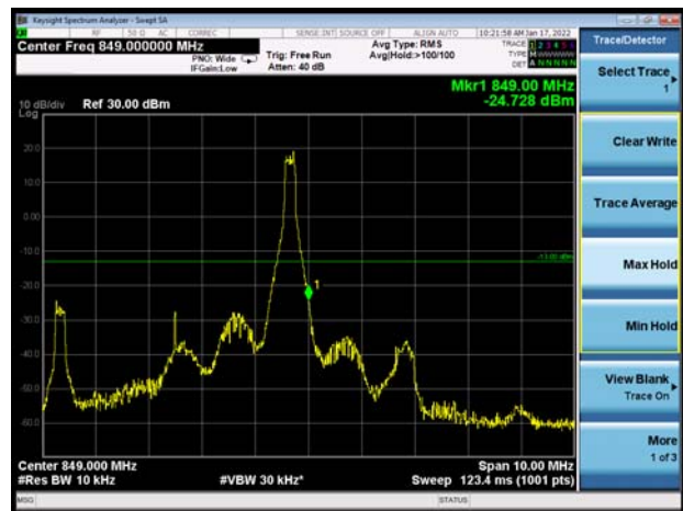
LTE Band 26 QPSK 5MHz CH-High 100%RB
