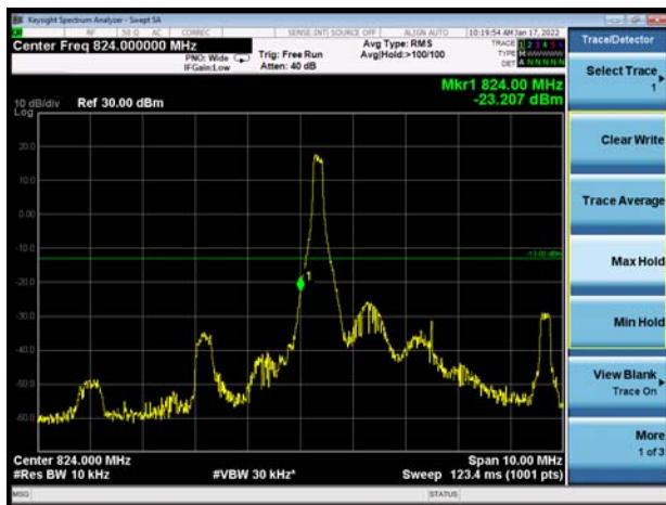
LTE Band 26 QPSK 5MHz CH-Low 100%RB
