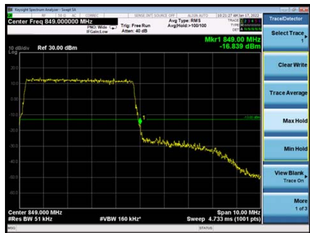
LTE Band 26 QPSK 5MHz CH-High 100%RB
