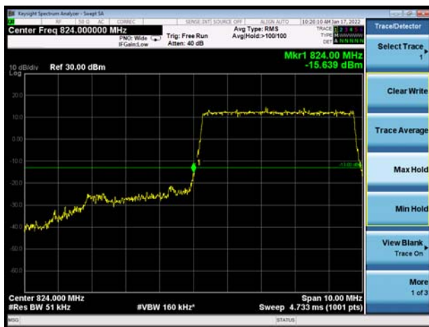
LTE Band 26 QPSK 5MHz CH-Low 100%RB
