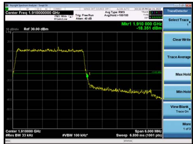
LTE Band 2 5MHz QPSK 1RB CH-High
