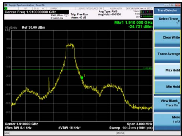
LTE Band 2 1.4MHz QPSK 100%RB CH-High
