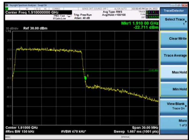
LTE Band 2 20MHz 16QAM 1RB CH-High
