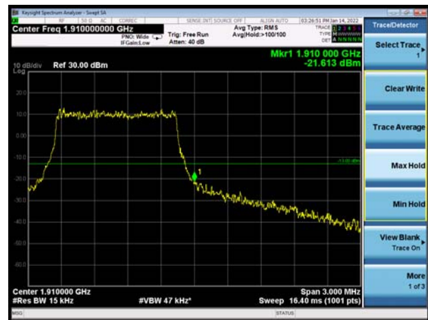
LTE Band 2 3MHz 16QAM 1RB CH-High
