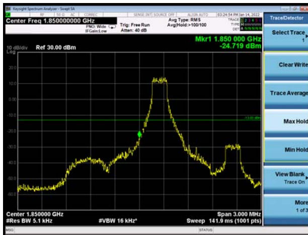
LTE Band 2 1.4MHz 16QAM 100%RB CH-Low
