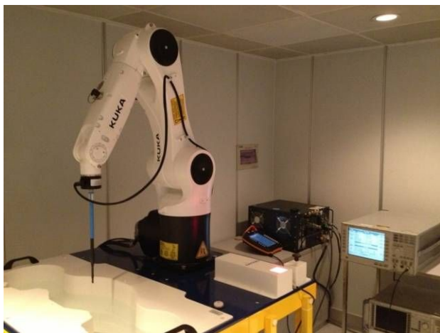
Photo 1: Measurement System SATIMO
