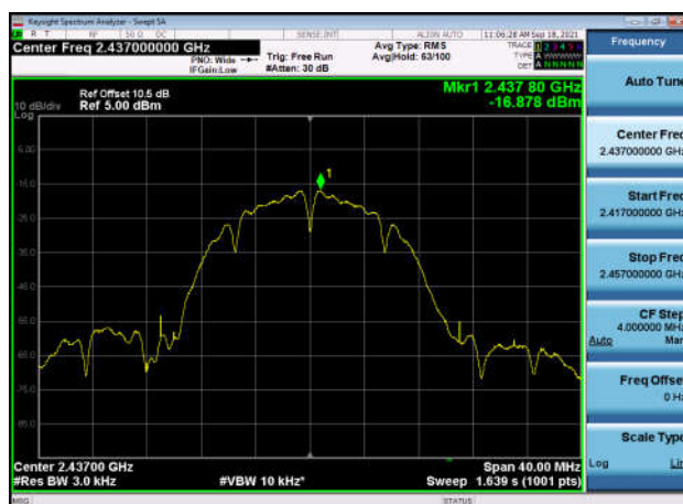
Power spectral density-802.11g ,2412MHz,Ant0
