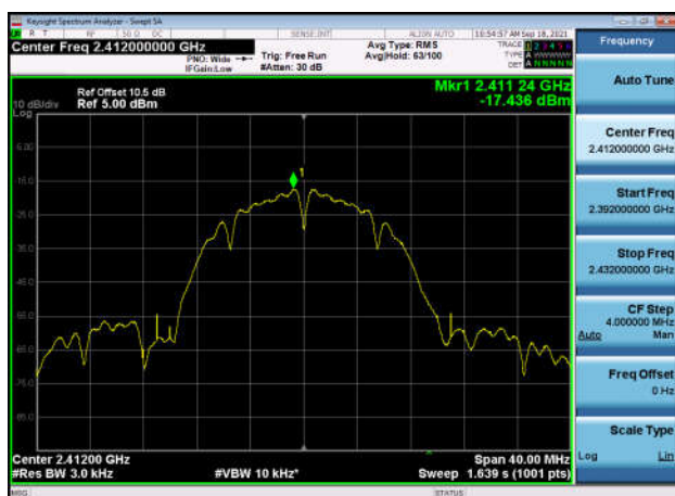
Power spectral density-802.11b ,2462MHz,Ant0
