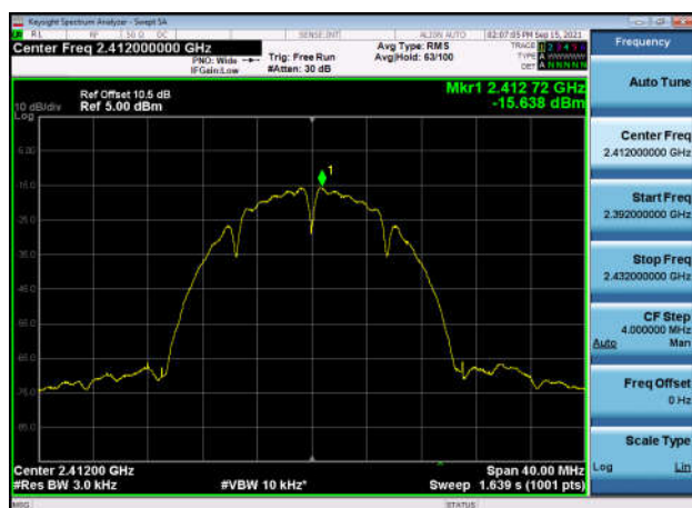
Power spectral density-802.11b ,2462MHz,Ant0
