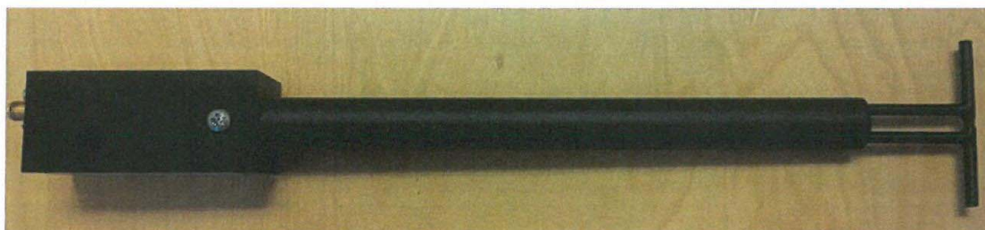
Figure 1 – MVG COMOSAR Validation Dipole
