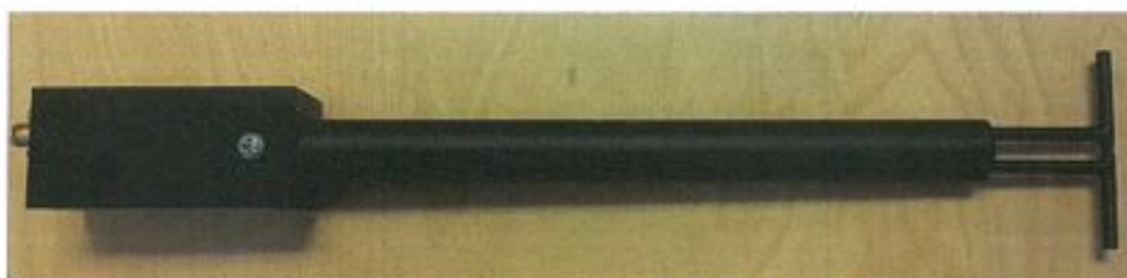
Figure 1 – MVG COMOSAR Validation Dipole
