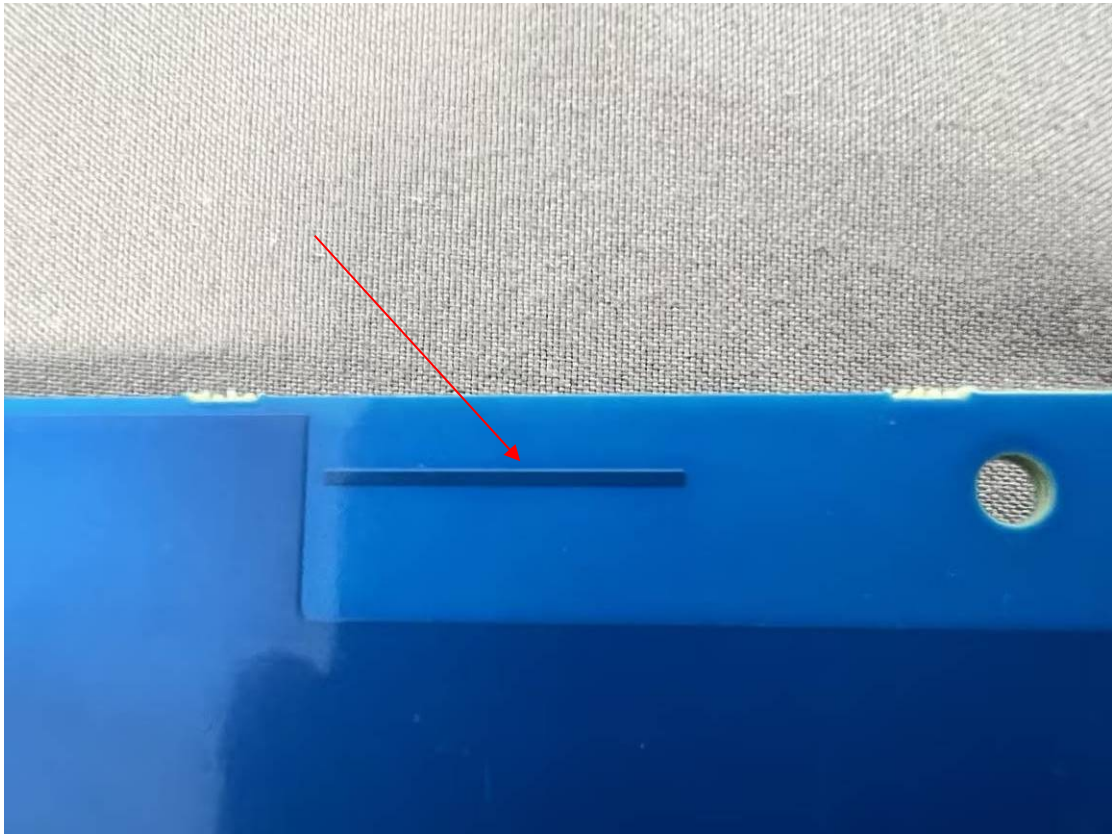
WIFI Antenna-Rear Side View
