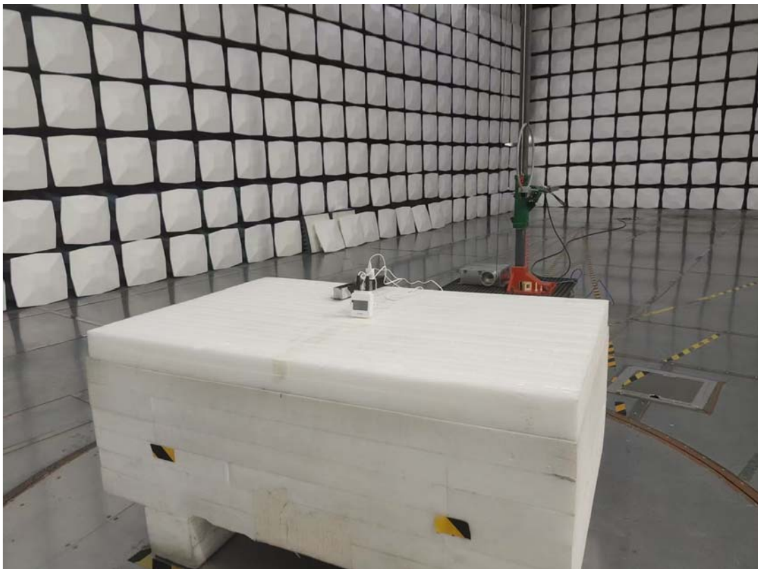
Radiated Emission 9k-30MHz Perpendicular View
