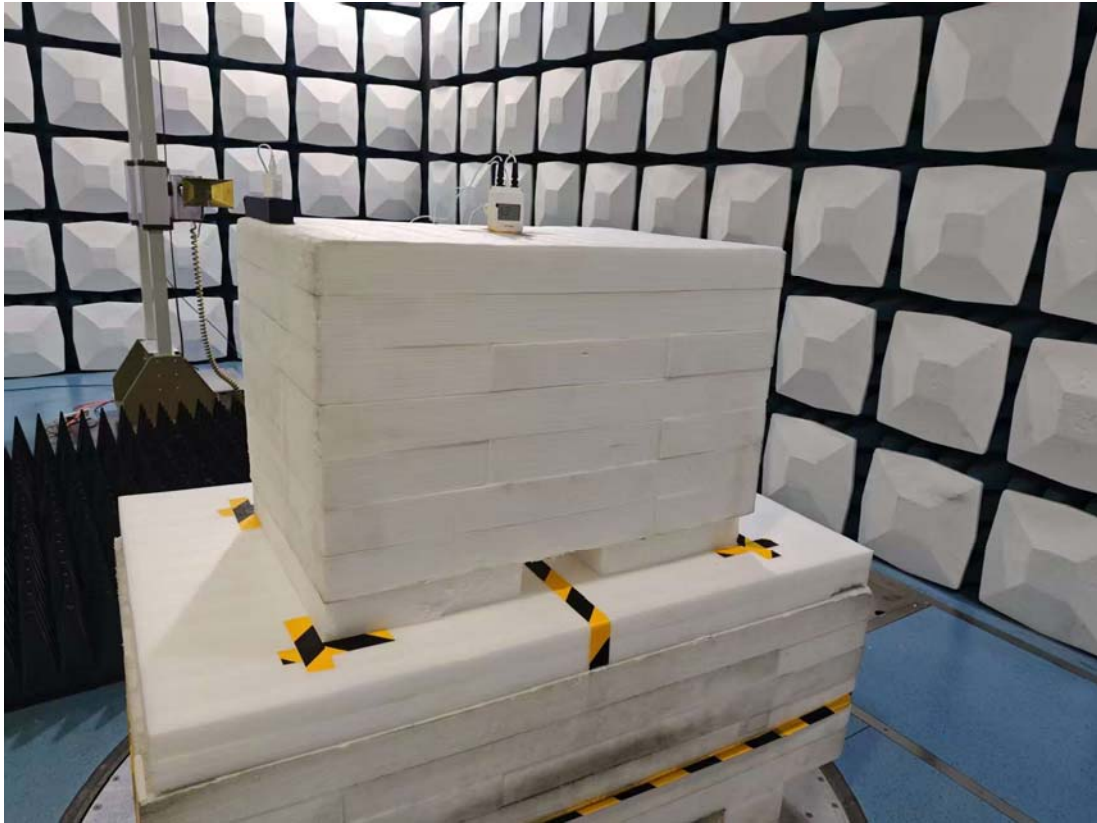
Radiated Emission Above 1GHz View
