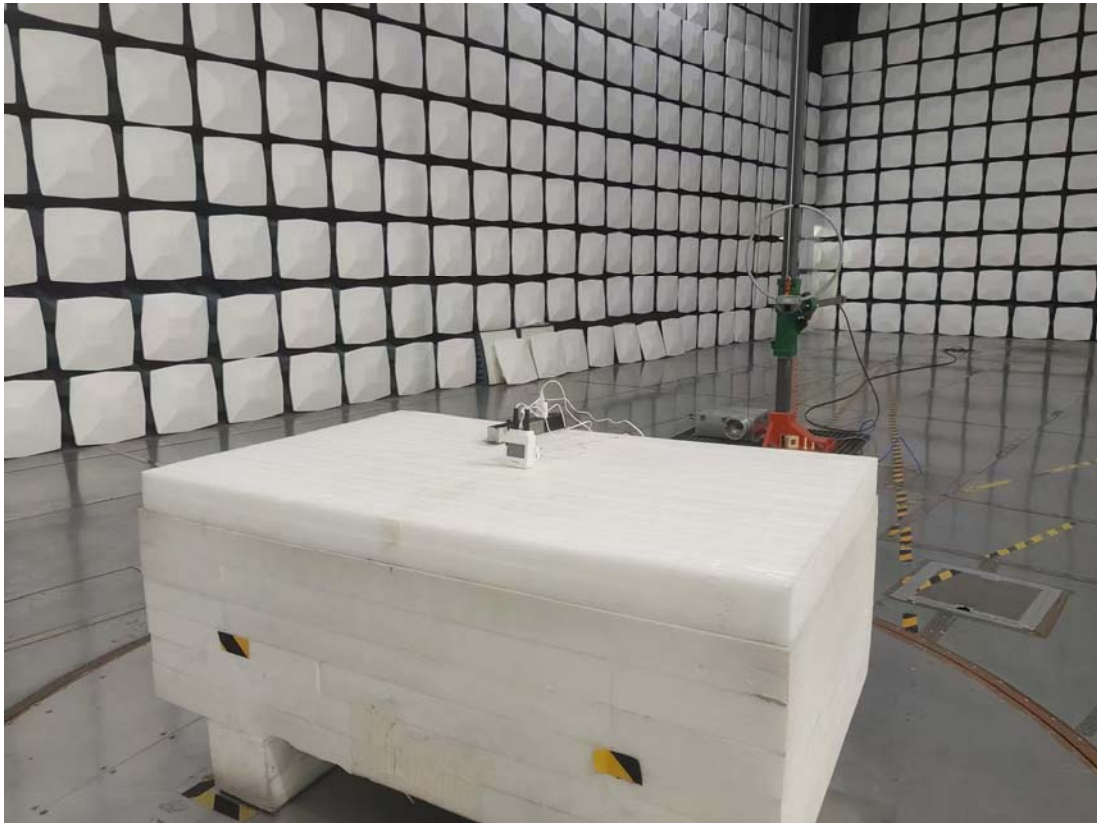
Radiated Emission 9k-30MHz Perpendicular View
