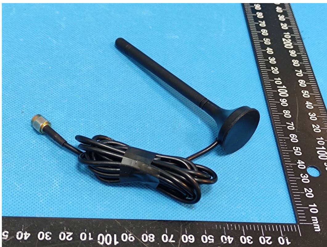
External Lora Antenna 2
