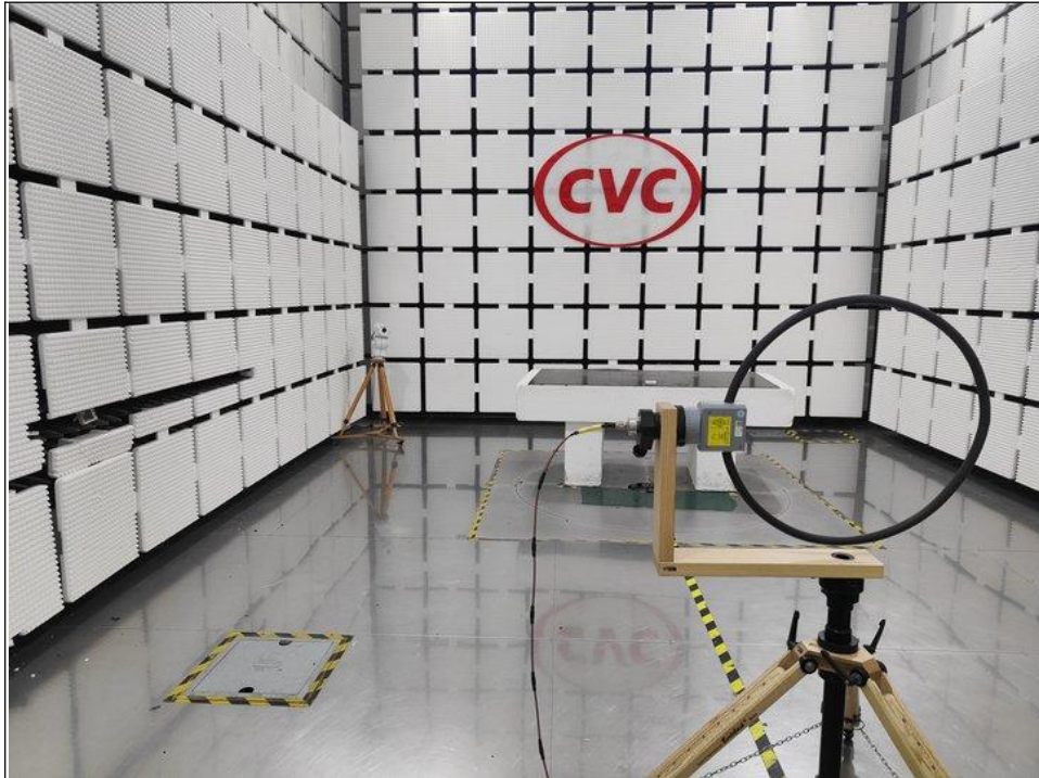
RADIATED EMISSION TEST (90KHz ~ 30MHz)
