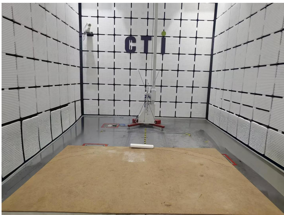
Radiated spurious emission Test Setup-1(Below 1GHz)
