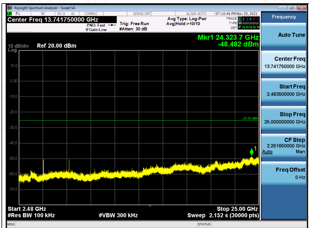
Test_Graph_BR_ANT1_2402_1Mbps_Higher Band Emissions
