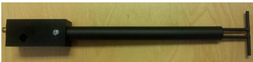
Figure 1 – MVG COMOSAR Validation Dipole
