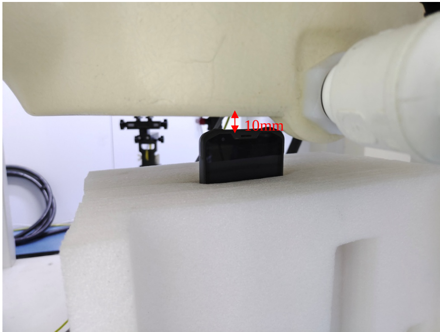
Body Top Setup Photo (10mm)
