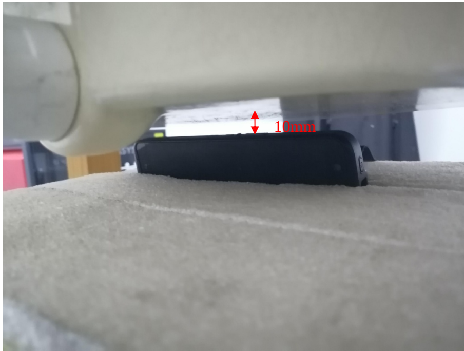
Body Right Setup Photo (10mm)
