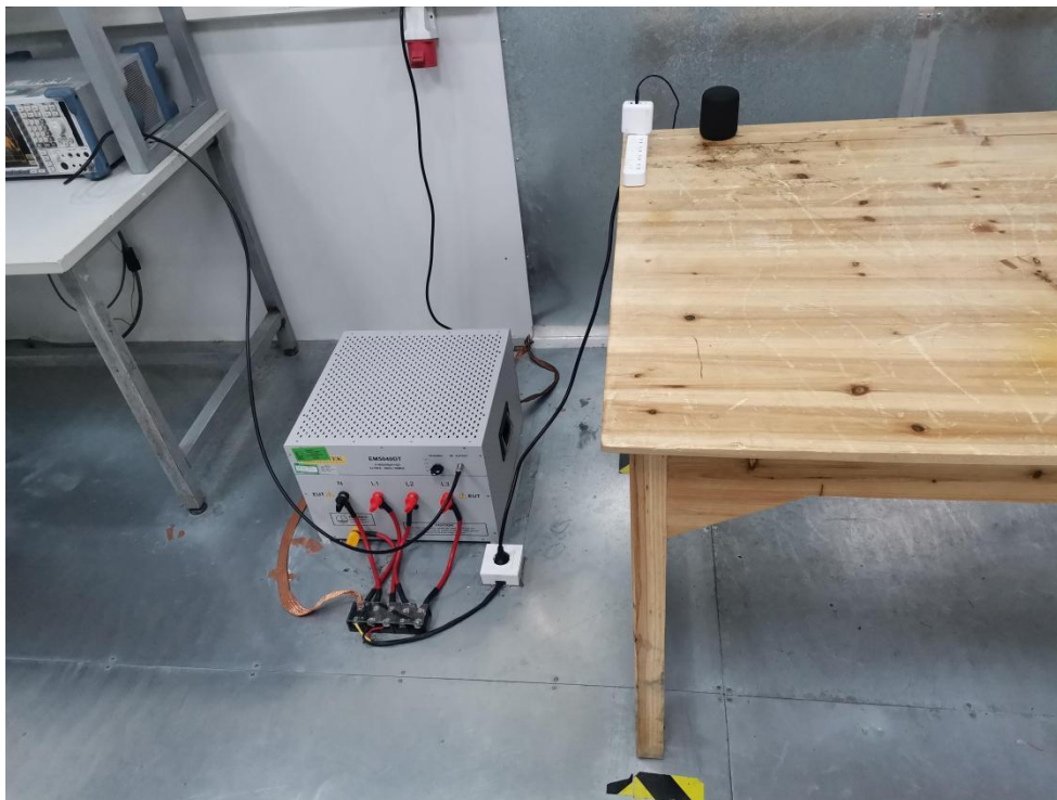
Photo of Conducted Emission Measurement
