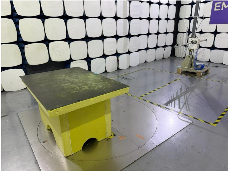
Spurious Emission Test Setup (Above 1GHz)
