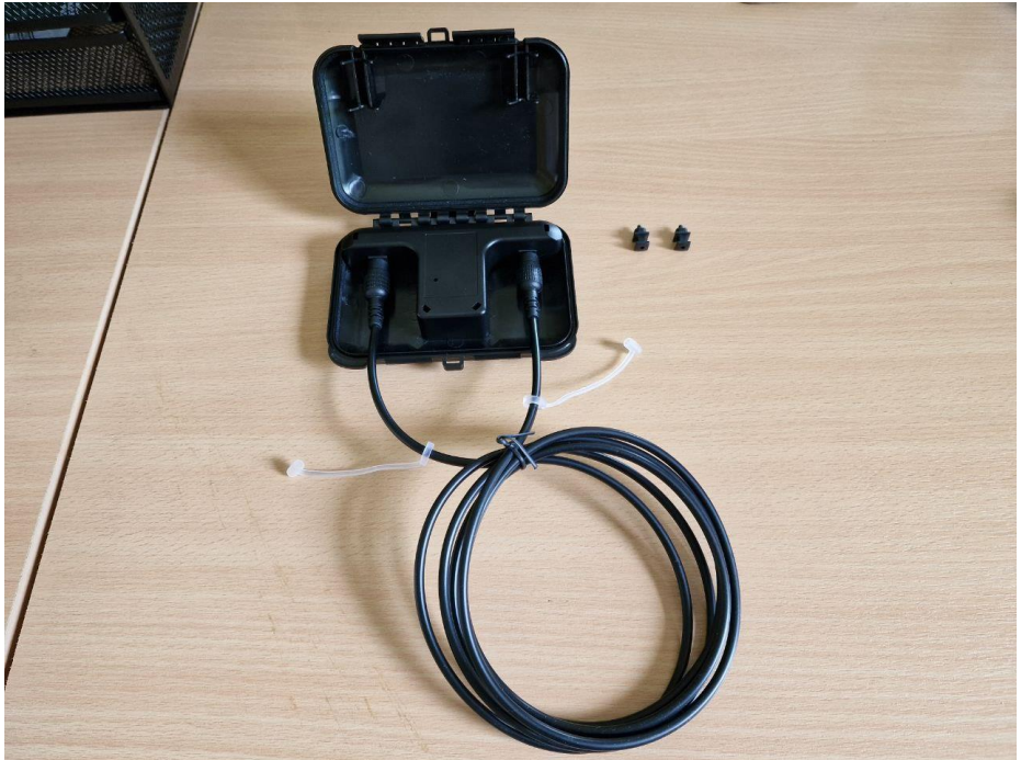
T1B device with its optical cable attached.
