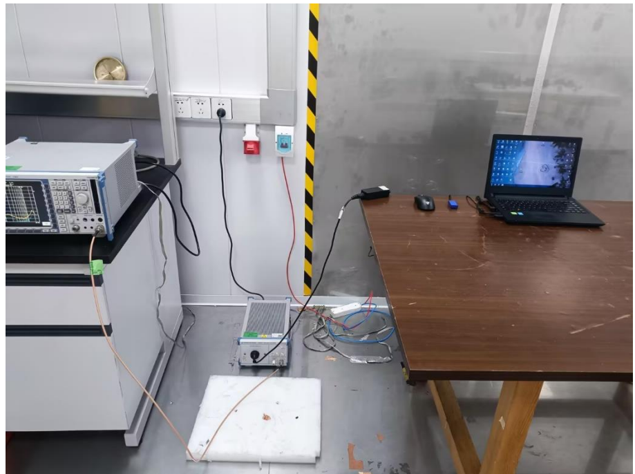
Conducted Emission Test Setup
