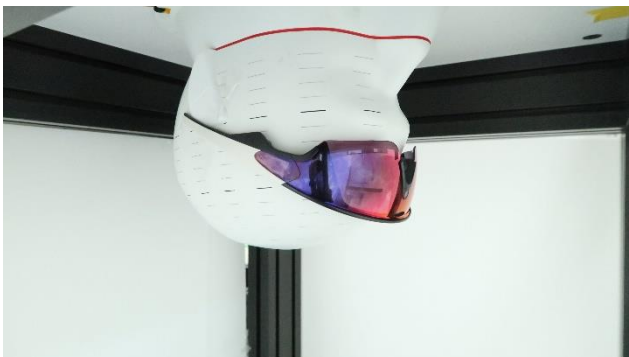
Rest-on-Head at 0mm
